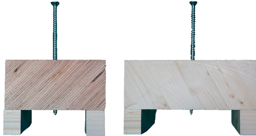
Figure 1. Timber products tested: Beech-LVL (left) and GLT from spruce ( Picea albies ) (right) with different load-to grain angles (45° (left) and 30° (right)).
