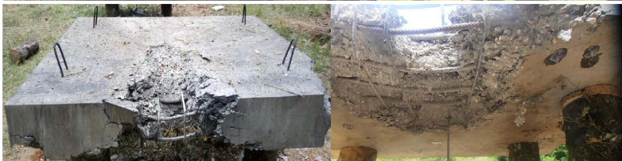
Figure 4. RC slab samples (RCS1-6) after explosive action: upper (left) and lower (right) surfaces.
