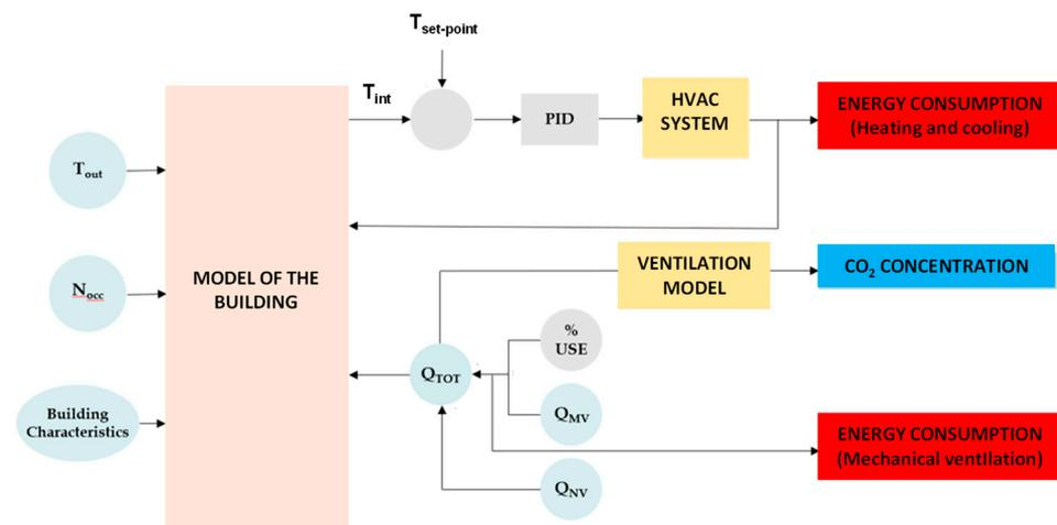
**Figure 14.** A possible scheme for the control of HVAC plants based on use of monitoring data.
