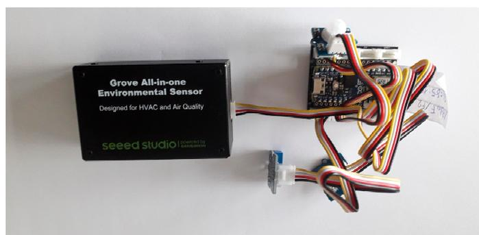
**Figure 4.** Multicomposed sensor obtained with Arduino ESP connected with specific sensors.
