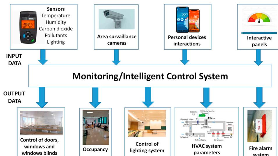
**Figure 1.** Monitoring data and their possible use for the smart control of the structure.
