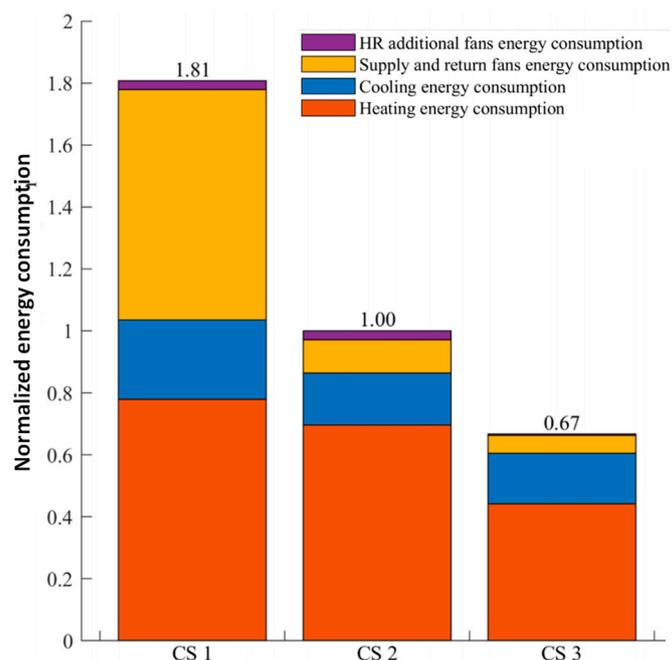
**Figure 15.** Normalized energy consumption with DCV strategies (CS3) with respect to a normal strategy (CS2) based on time operation and COVID-19 (CS1) in the structure of Figure 6a.
