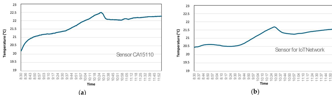
**Figure 5.** Comparison of temperature measurement in the same position: data from a typical analogic sensor (a) and a modern sensor for an IoT network (b).
