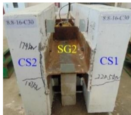
(a) SG2 side view of the D16C30 specimen
