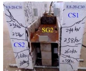
(b) SG2 side view of the D20C30 specimen
