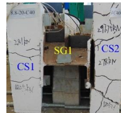
(c) SG1 side view of the D20C40 specimen
