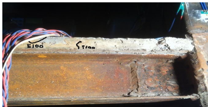
Figure 10. Cracks in the floor of SJ1 model.
