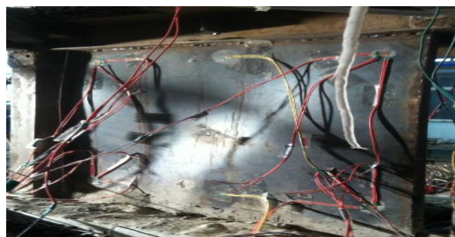
Figure 13. Shear wall tension band of SJ2 model.
