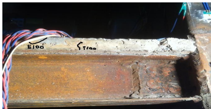
Figure 10. Cracks in the floor of SJ1 model.
