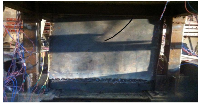
Figure 11. Shear wall tension band of SJ1 model.
