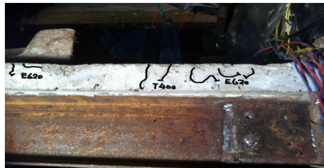
Figure 12. Cracks in the floor of SJ2 model.
