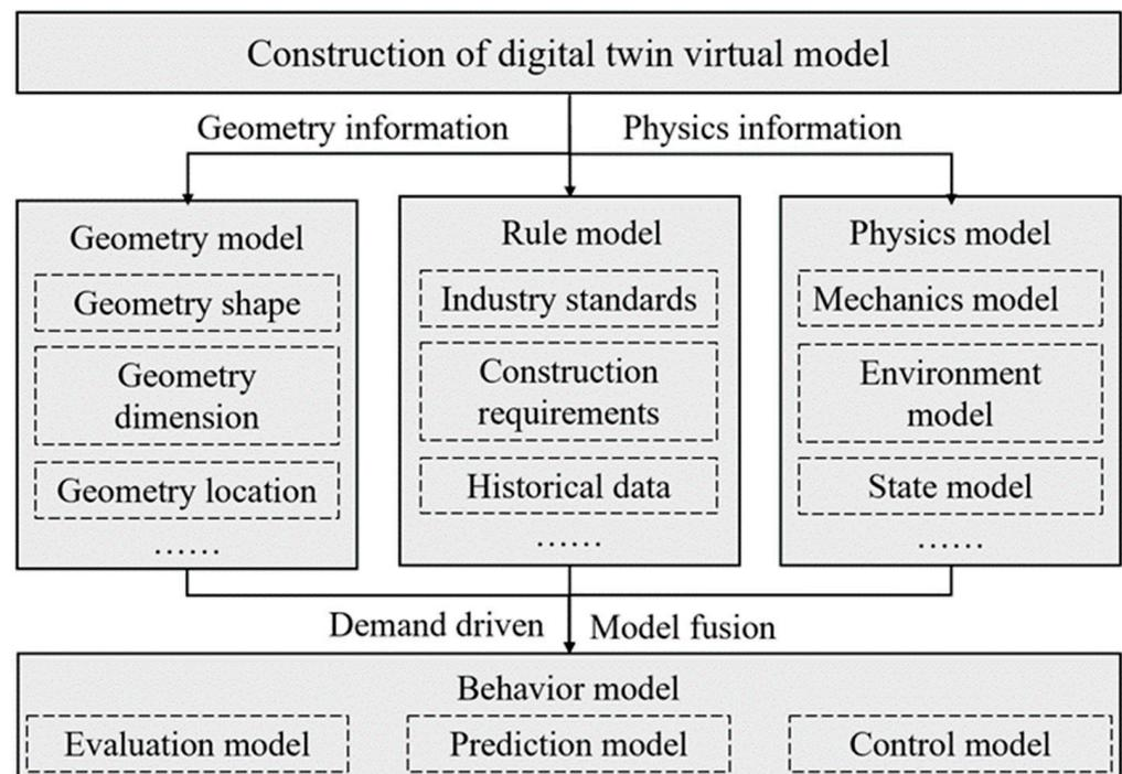
**Figure 4.** Construction of a digital twin virtual model.
