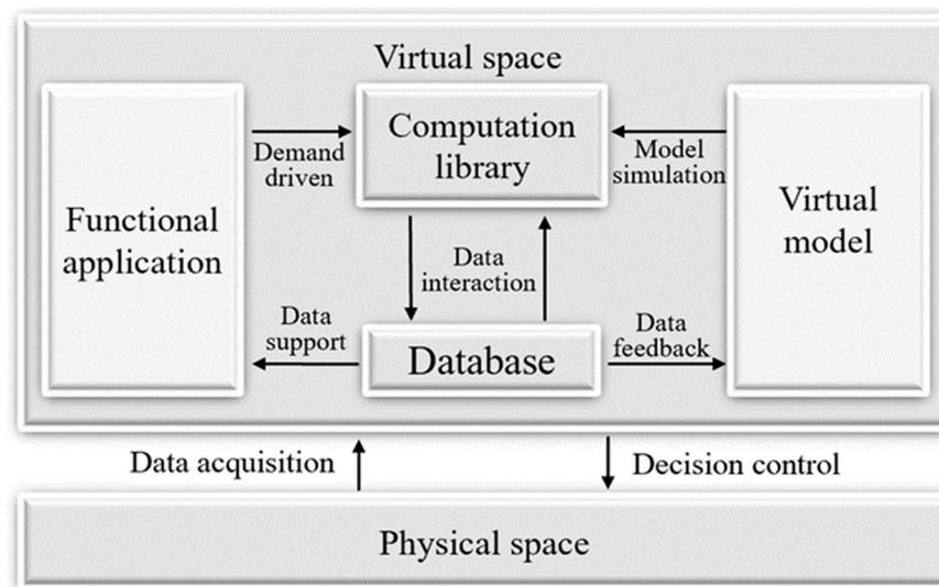
**Figure 5.** Information exchange of the digital twin model.
