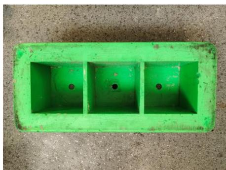
Figure 3. Pictures of the plastic molds.
