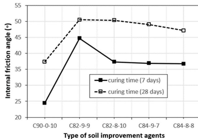
Figure 6. Friction angle variation of mixture.
