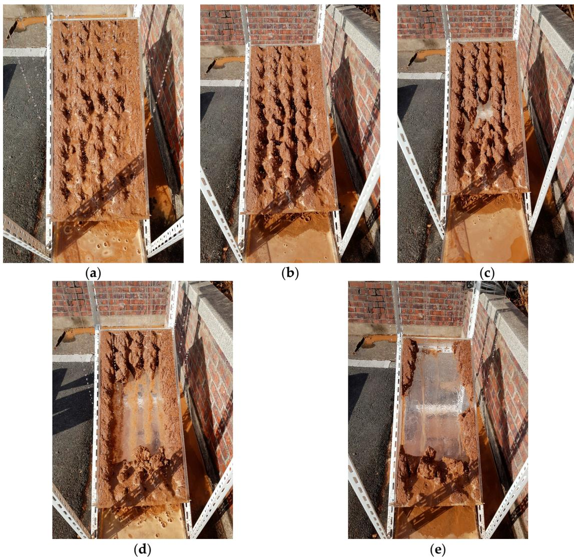
**Figure 8.** Erosion test due to rainfall with various times (original soil: C-90-0-10). (a) 5 min after rainfall; (b) 10 min after rainfall; (c) 15 min after rainfall; (d) 20 min after rainfall; (e) 30 min after rainfall.
