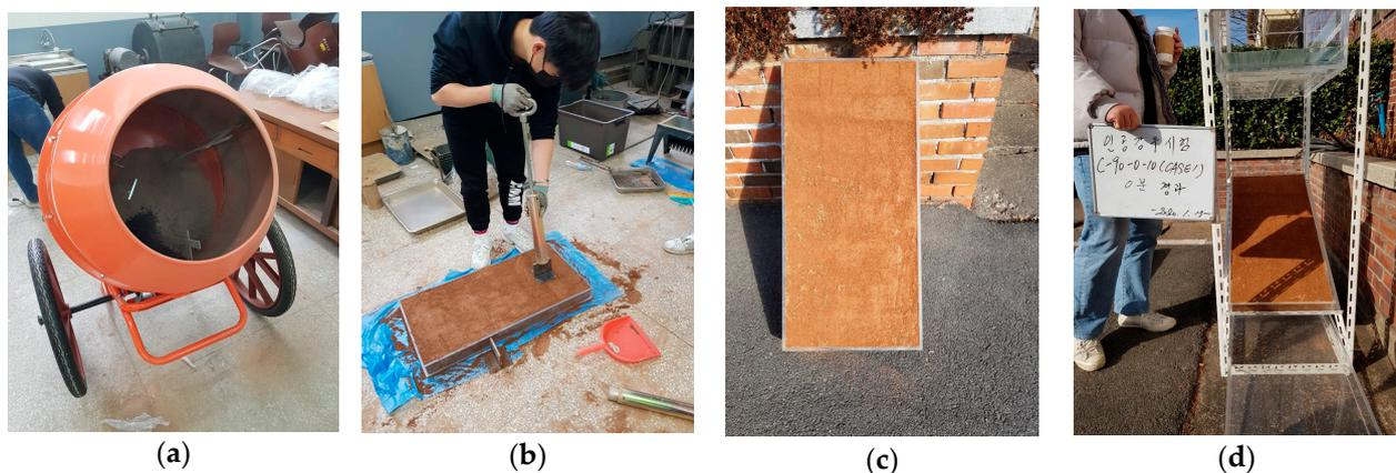
Figure 7. Experimental procedure for soil slope erosion test by rainfall. (a) mixing process of samples; (b) compaction of soil mixture; (c) curing time by type; (d) slope frame set for rainfall test.
