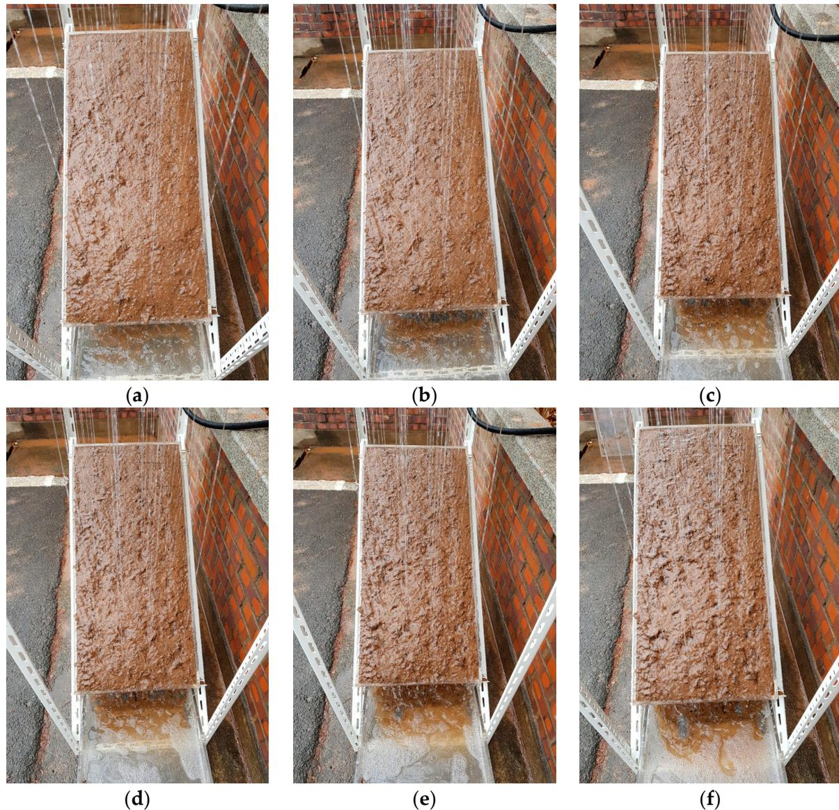
**Figure 9.** Erosion test due to rainfall with various times (mixed soil: C-82-9-9). (a) 5 min after rainfall; (b) 10 min after rainfall; (c) 20 min after rainfall; (d) 30 min after rainfall; (e) 40 min after rainfall; (f) 60 min after rainfall.
