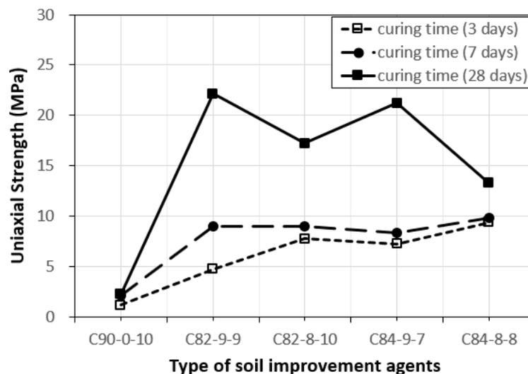
**Figure 4.** Uniaxial compressive strength of mixed soils.
