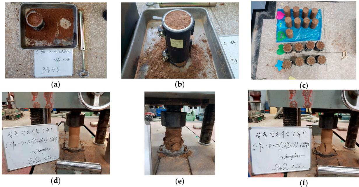
**Figure 3.** Sample preparation and uniaxial compression test. (a) Mixture preparation; (b) compaction of soil mixture; (c) soil mixture with curing time; (d) uniaxial compression test; (e) failure of uniaxial test; (f) measurement by type.
