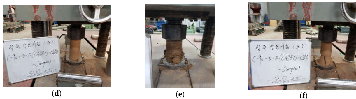
Figure 3. Sample preparation and uniaxial compression test. (a) Mixture preparation; (b) compaction of soil mixture; (c) soil mixture with curing time; (d) uniaxial compression test; (e) failure of uniaxial test; (f) measurement by type.
