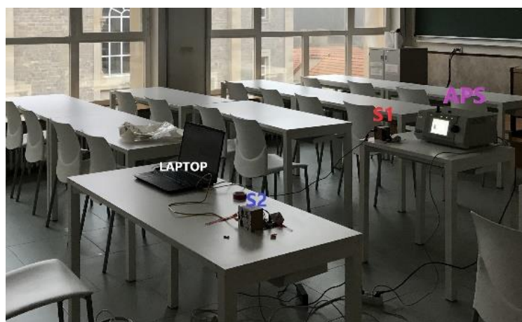
Figure 2. Example instrument layout in University Classroom A206. S1 and S2 are the SCD30 sensors; APS is the aerodynamic particle sizer and laptop (hardware for instrument data storage).
