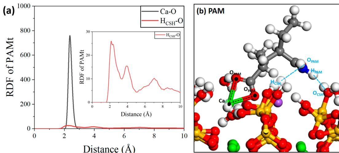
**Figure 20.** (a) RDF of PAM/C-S-H and (b) local structure.
