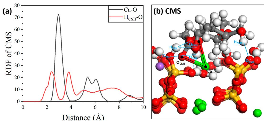
**Figure 17.** (a) RDF of CMS/C-S-H and (b) local structure.
