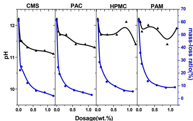
**Figure 6.** The mass loss and pH of cement paste with different AWAs. (The black lines represent changes in pH value, while the blue lines represent changes in mass loss).
