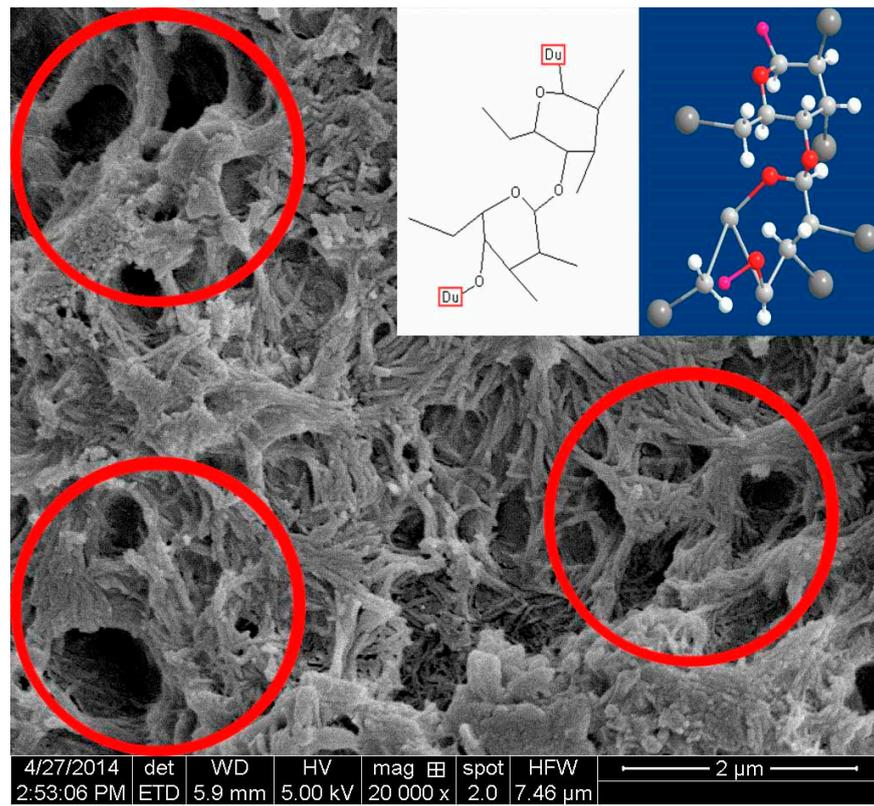
Figure 9. Scanning electron micrograph of the dried cement paste with HPMC.
