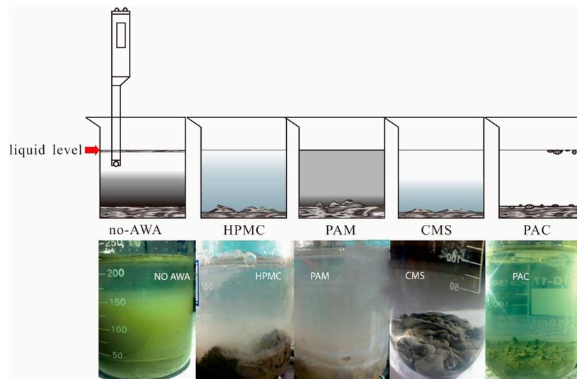
**Figure 3.** Flocculation states of cement paste with different AWAs.
