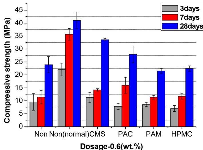
**Figure 14.** The compressive strength of UWC at an AWCA dosage of 0.6%.
