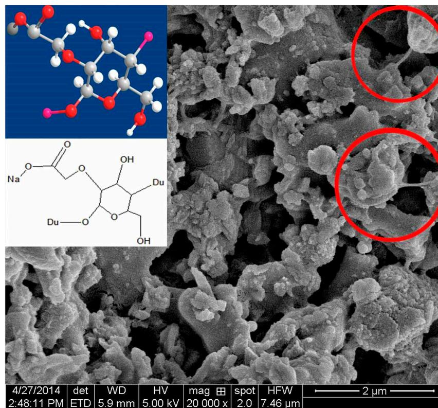
Figure 8. Scanning electron micrograph of the dried cement paste with CMS.
