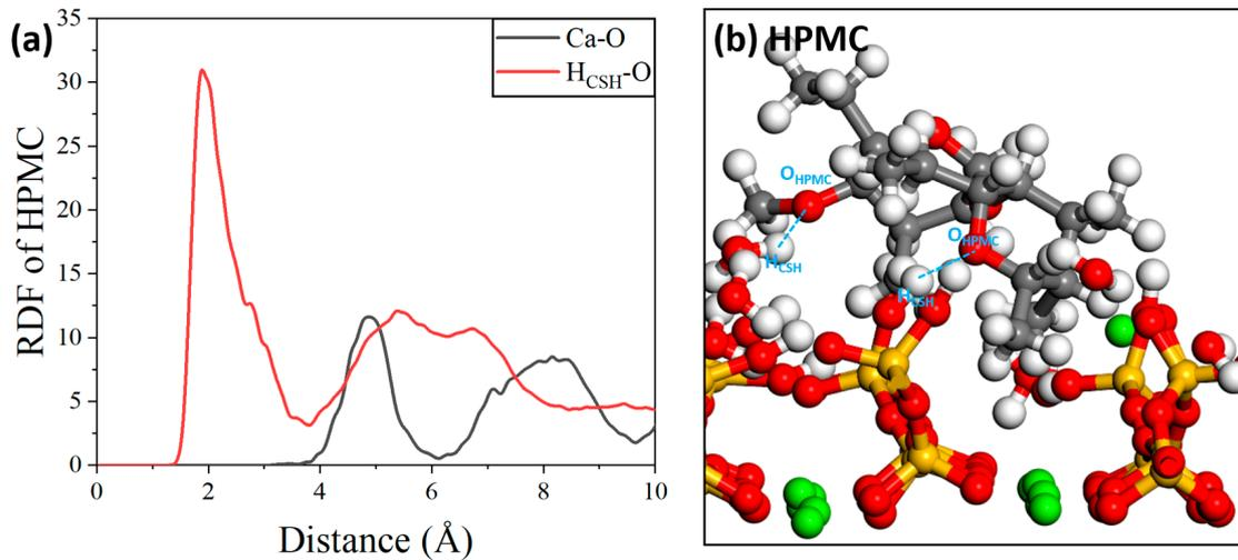
**Figure 18.** (a) RDF of HPMC/C-S-H and (b) local structure.
