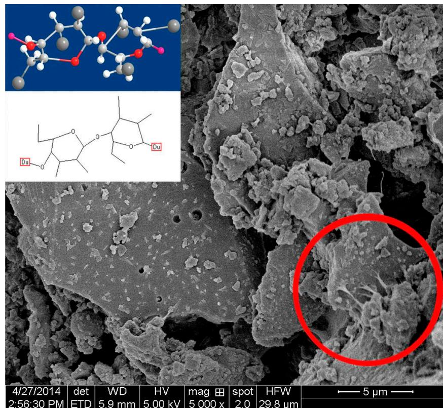
Figure 10. Scanning electron micrograph of the dried cement paste with PAC.
