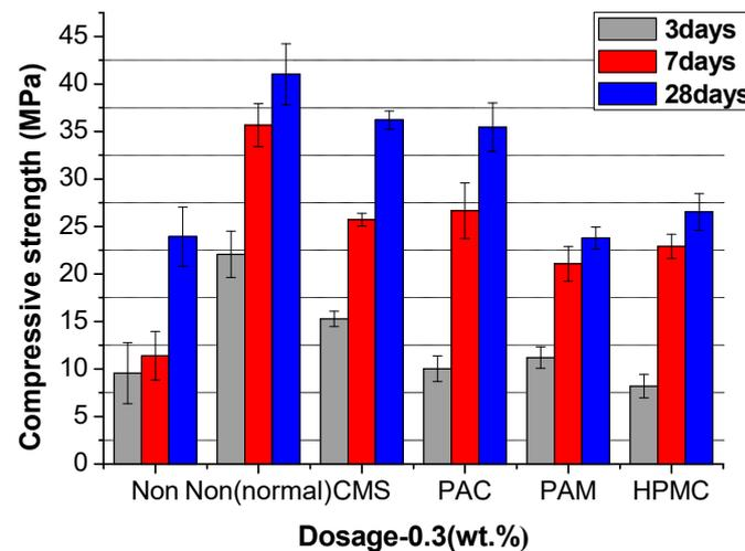
Figure 13. The compressive strength of UWC at an AWCA dosage of 0.3%.
