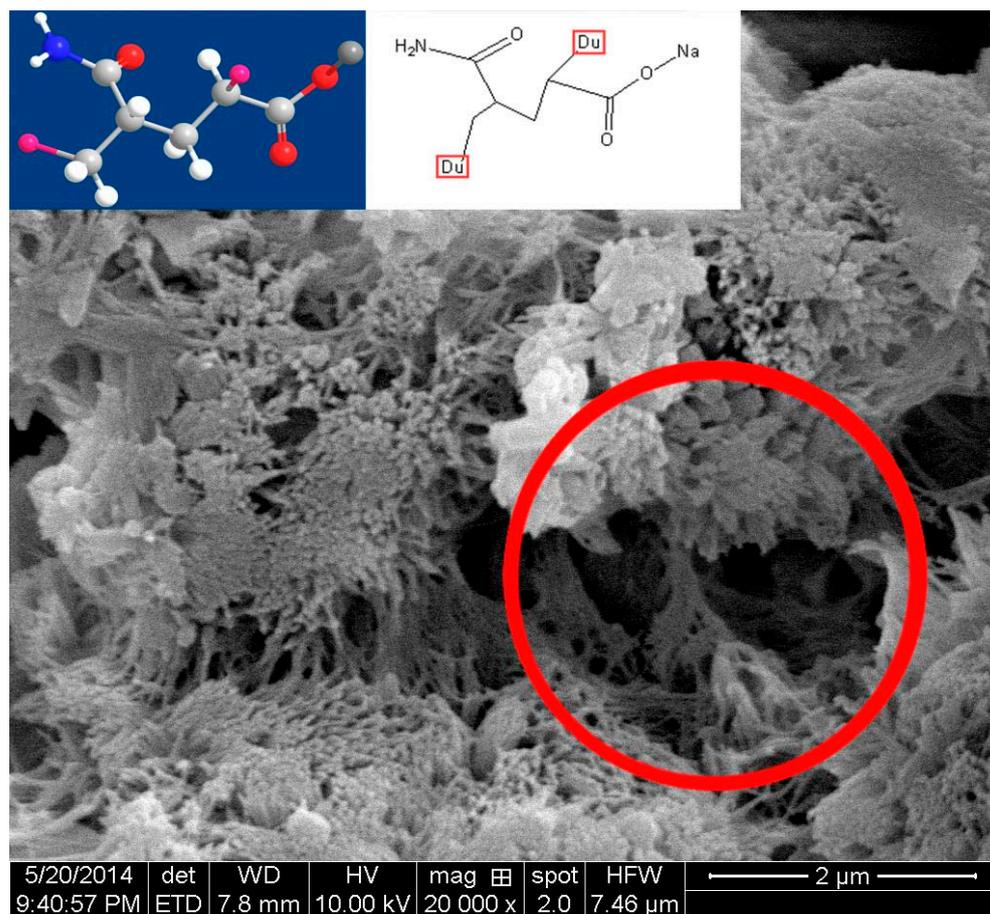
**Figure 11.** Scanning electron micrograph of the dried cement paste with PAM.
