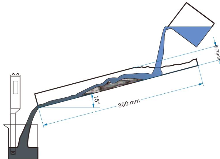
Figure 5. Stream test.
