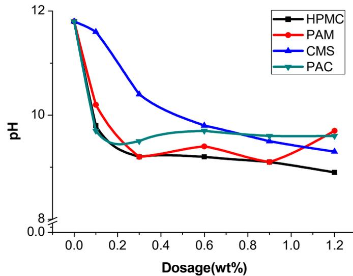
Figure 4. pH of the supernatant solution with different AWAs.
