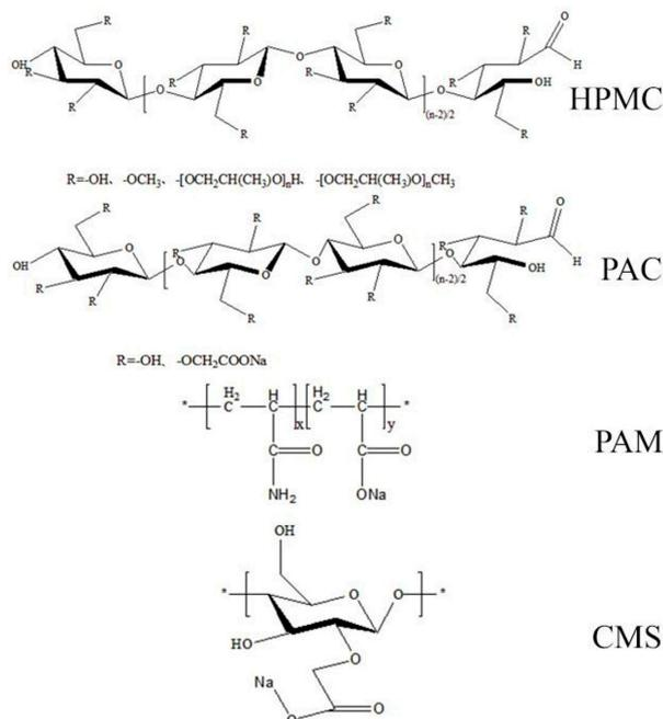
**Figure 15.** Chemical formulas of different AWAs. (The position of \* means the starting and ending segments of each polymer repeating segment).
