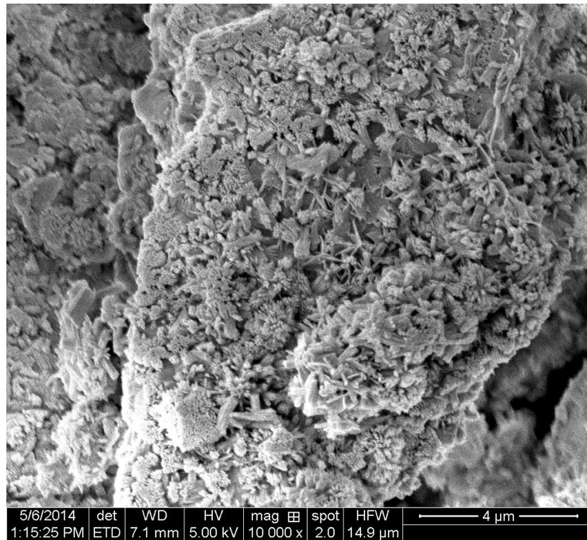
Figure 7. Scanning electron micrograph of the dried cement paste without AWAs.
