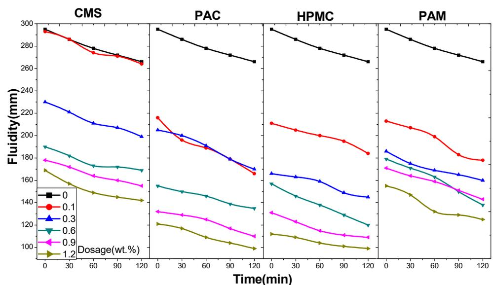
Figure 1. Fluidity and fluidity loss of cement paste with CMS, PAC, HPMC, and PAM.
