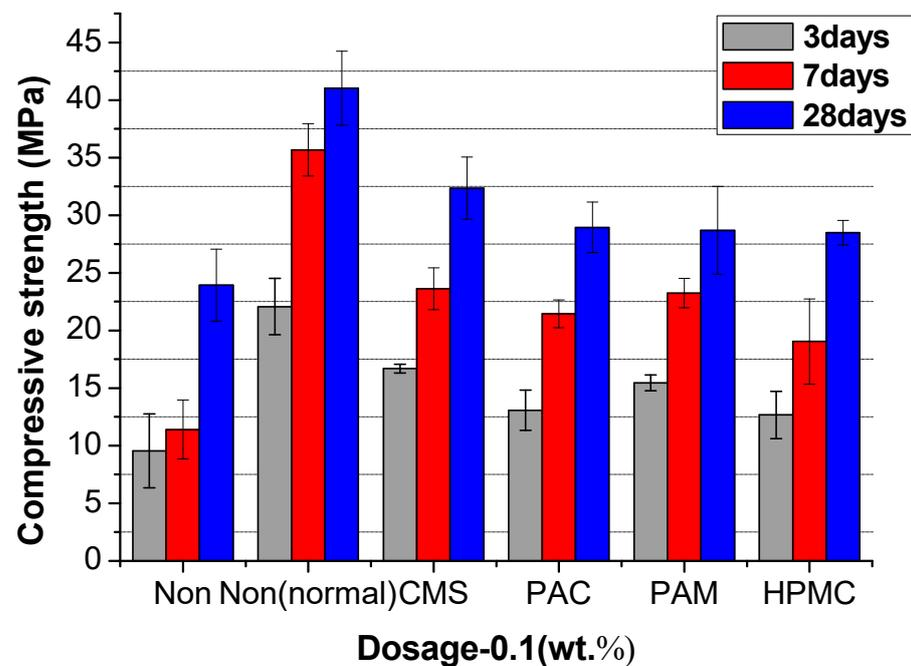
Figure 12. The compressive strength of UWC at an AWCA dosage of 0.1%.
