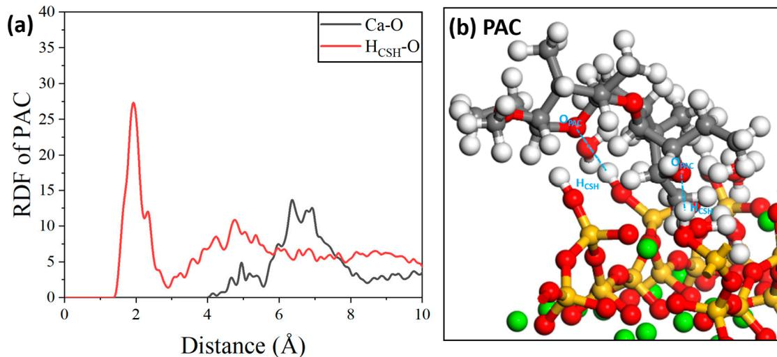
**Figure 19.** (a) RDF of PAC/C-S-H and (b) local structure.
