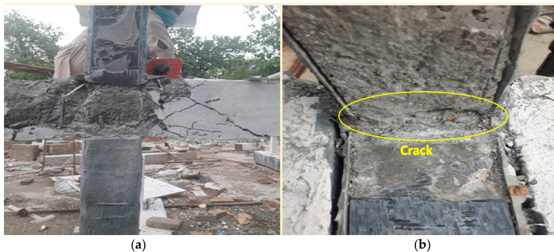
Figure 11. Undamaged concrete, (a) in joint covered by CFRP laminate, and (b) above joint covered by L-shaped CFRP sheets.
