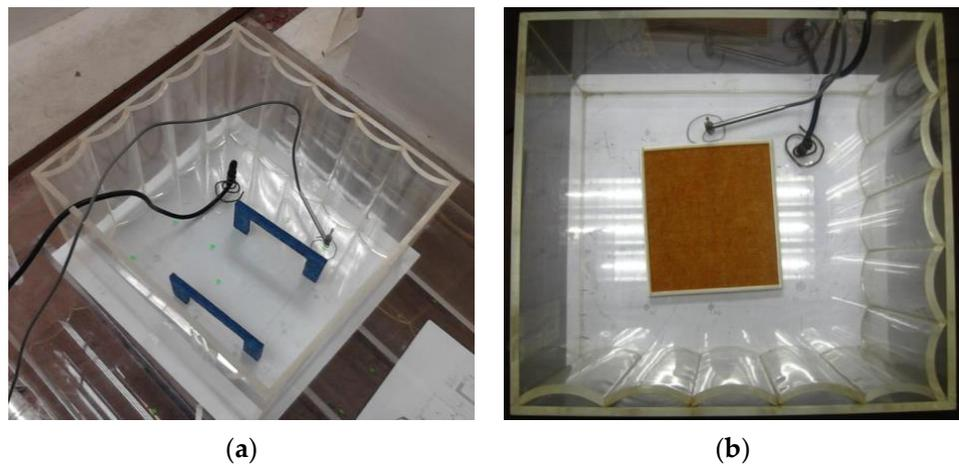
**Figure 11.** Photos of absorption coefficient measurements in the 1:20 scaled reverberation chamber: (a) “stage curtains”; (b) polyester fiber board.
