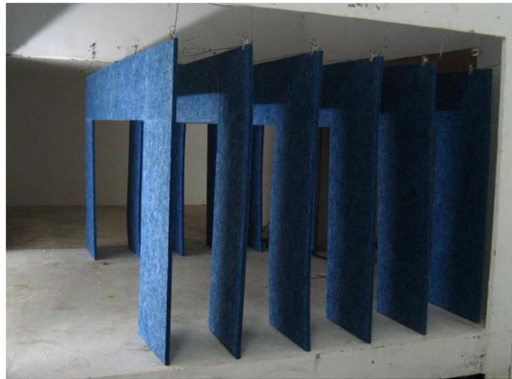
**Figure 10.** Photo of stage curtains for scaled model measurements.
