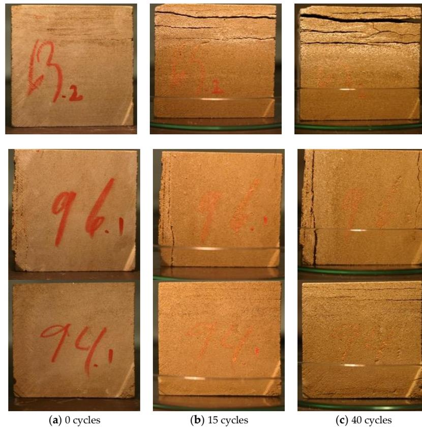
**Figure 6.** Detailed aspects of three representative specimens before and after the sodium chloride crystallization–dissolution test.
