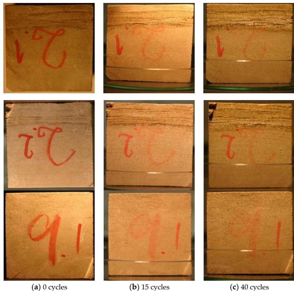
**Figure 10.** Detailed aspects of three representative specimens before and after the sodium sulfate crystallization and dissolution cycles.
