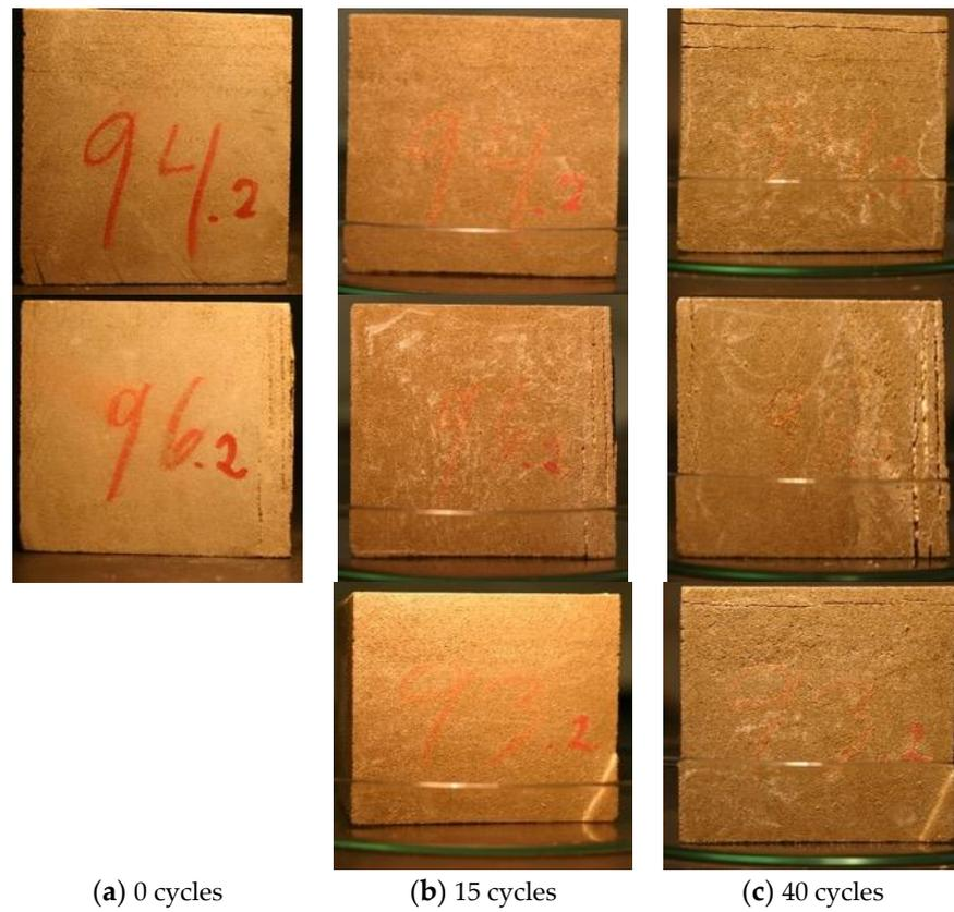
**Figure 7.** Detailed aspects of three representative specimens before and after the crystallization and dissolution cycles of sodium chloride and calcium sulfate solution.
