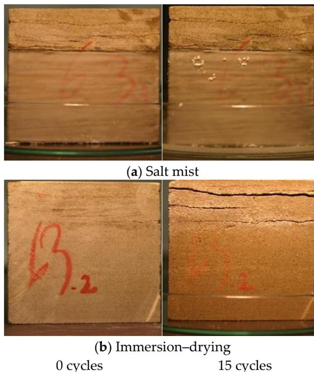
**Figure 4.** Aspect of specimens after salt crystallization tests by: (a) salt mist; (b) immersion/drying (left and right columns correspond to 0 and 15 cycles).
