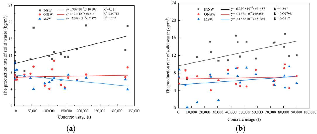
**Figure 5.** Effect of the amount of concrete usage on solid waste generation rate. (a) Office buildings; (b) Exhibition buildings.
