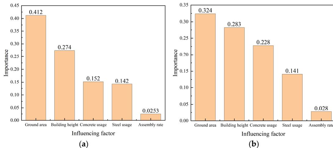
**Figure 2.** Importance analysis of factors affecting solid waste generation rate at construction sites. (a) Office buildings; (b) Exhibition buildings.
