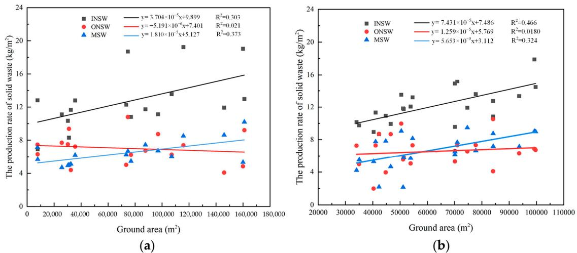
**Figure 3.** Effect of ground area on solid waste generation rate. (a) Office buildings; (b) Exhibition buildings.
