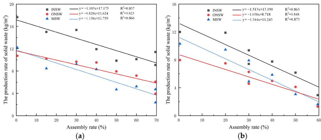
**Figure 7.** Effect of the assembly rate on solid waste generation rate. (a) Office buildings; (b) Exhibition buildings.
