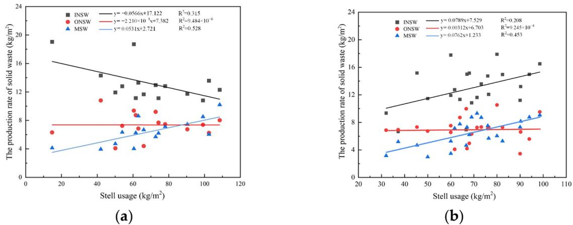
**Figure 6.** Effect of the amount of steel usage on solid waste generation rate. (a) Office buildings; (b) Exhibition buildings.
