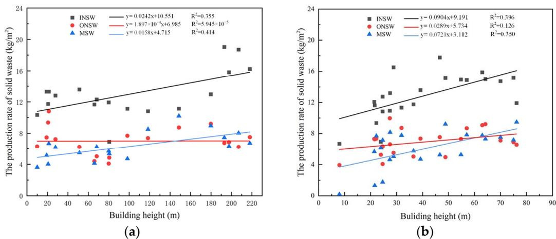
**Figure 4.** Effect of building height on solid waste generation rate. (a) Office buildings; (b) Exhibition buildings.
