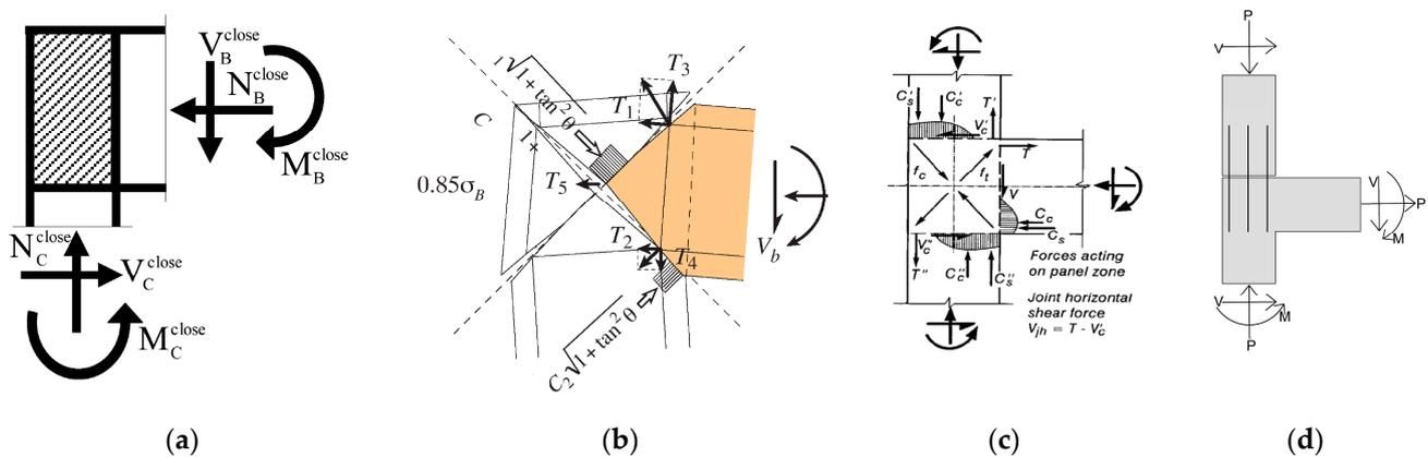
**Figure 13.** Cases of joints: (a) knee [41], (b) knee with internal forces [16], (c) external treated by internal forces [42], and (d) untreated hinge connection.
