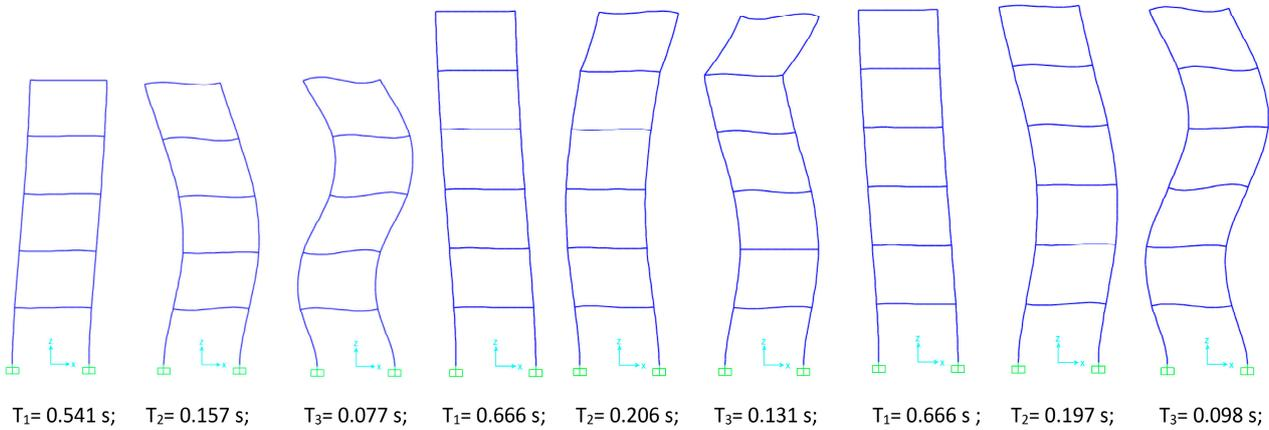
(D) New frame with 5+2 added floor stiff joint;      (E) New frame with 5+2 added floor hinge joint
