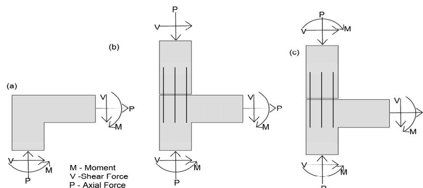
**Figure 4.** Column knee joint: (a) existing joint, (b) pinned connection, and (c) rigid connection.
