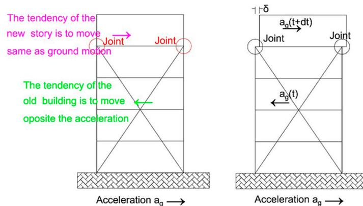
**Figure 5.** Tendency of the displacement of the added floor on the old building.
