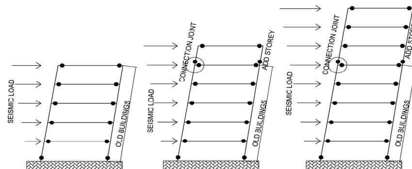
**Figure 6.** Display of the plastic cracks on the old building and the building with added floors.
