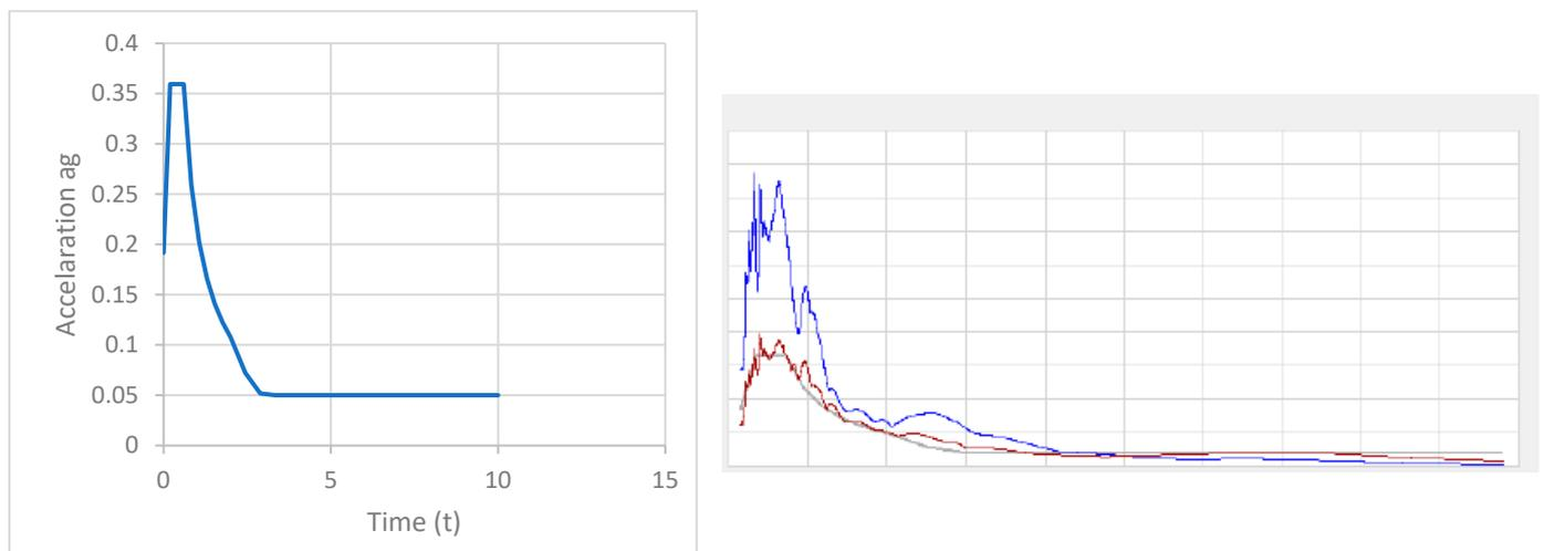
**Figure 11.** Respond spectrum and time history spectrum  $a_g(t)$ . The blue-colored curve represents the time history of the response spectrum for an acceleration of  $a_g = 0.4$  g, while the red-colored curve depicts the time history of the response spectrum for an acceleration of  $a_g = 0.25$  g.
