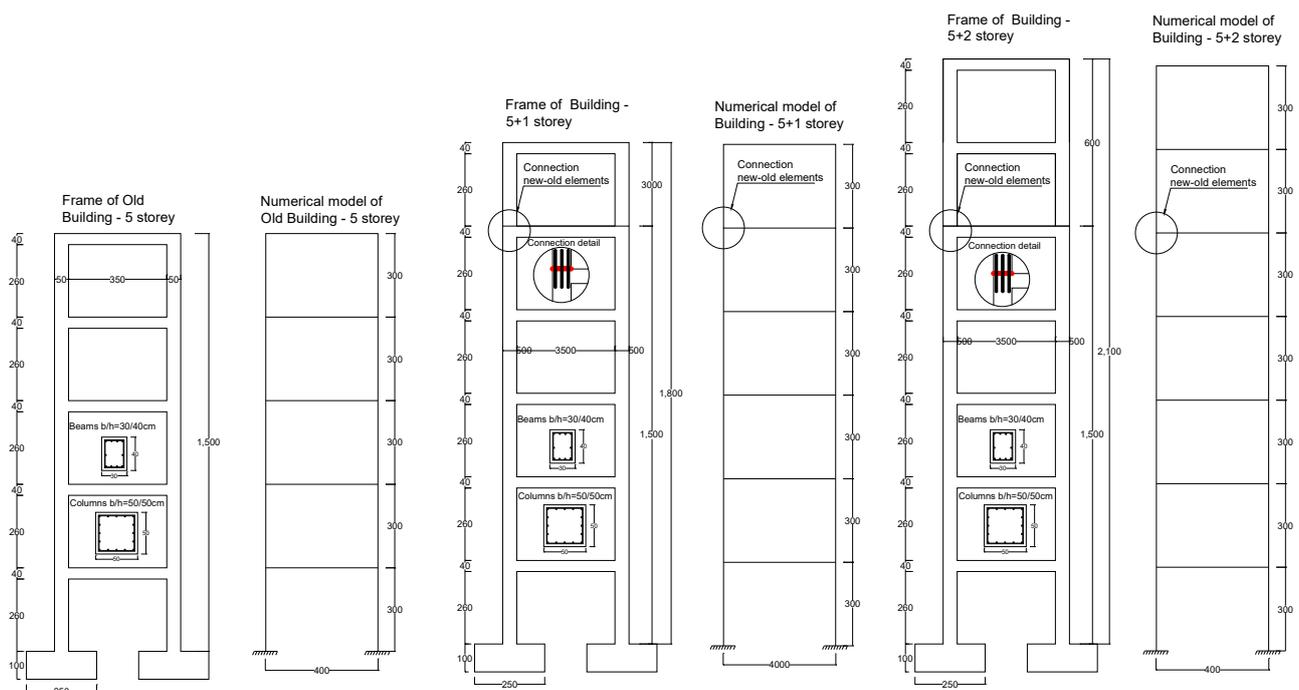
**Figure 9.** Numerical model and column and beam cross-sections of the old frame and the frames with additional floors.
