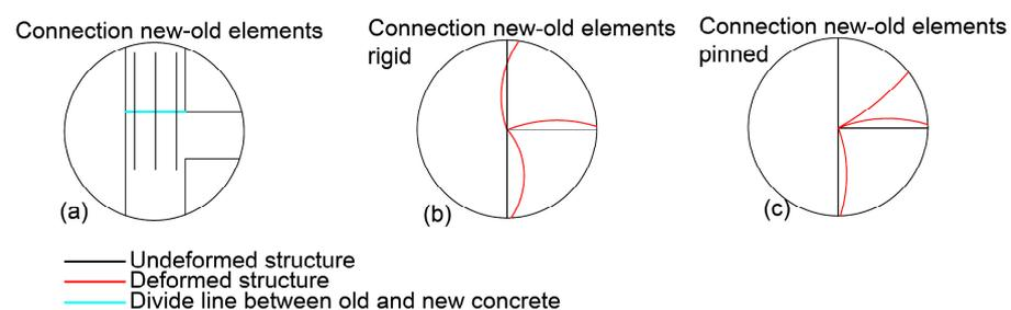
**Figure 12.** Connection at joint 6 and its deformation on rigid and hinged connections, (a) The executed connection of the supplementary column; (b) the form of deformation of the rigid connection; (c) the form of deformation of the hinge connection.
