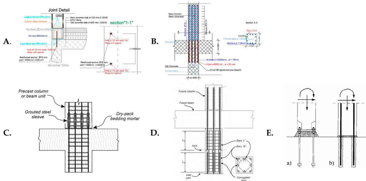
**Figure 3.** Several examples of connections executed in practice and from the literature (A,B) executed in Kosovo, ((C) [9], (D) [9], (E) [10]) for the addition of floors and prefabricated elements.
