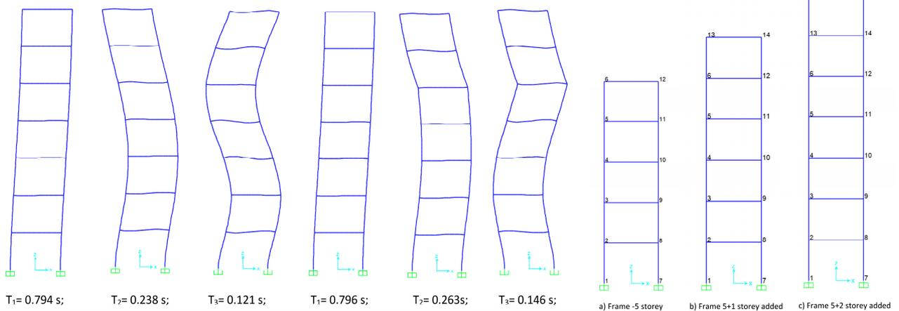
**Figure 10.** Periods and modes for the three models of base frames and frames with additional floors, as well as the undeformed models.
