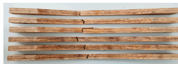
Figure 6. Failure state of bamboo scrimber tensile specimen.
