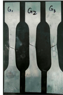
Figure 9. Failure state of steel tensile specimens.
