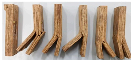
Figure 3. Failure state of bamboo scrimber compressive specimen.
