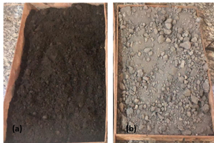
Figure 1. Steel slag used in this research. (a) In wet form; (b) in dry form.
