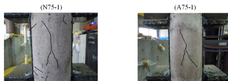
Figure 8. Cracks on inner concrete after test.
