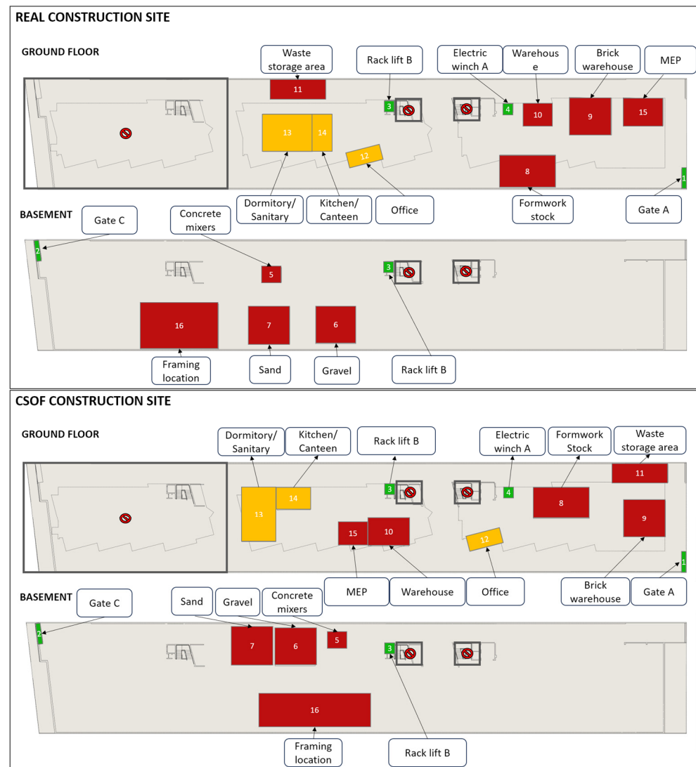
Figure 13. Visualization of construction sites in the third study. This figure presents the actual construction site layout at the top, showing how it was executed in practice, and the optimized layout generated by the framework at the bottom.
