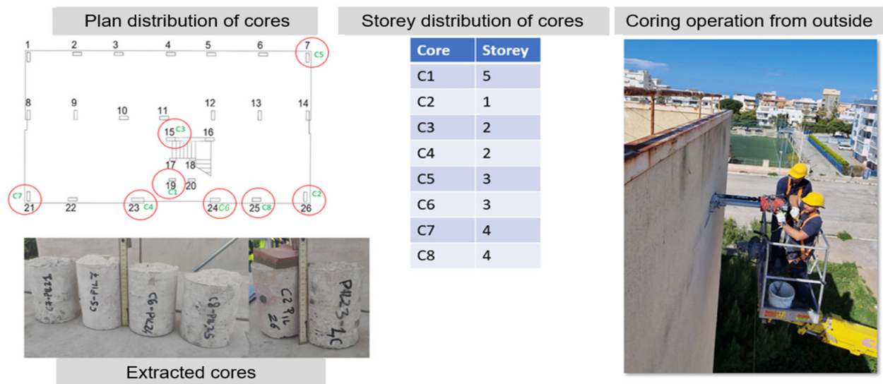
Figure 10. Concrete core drilling (for column and storey numbers, see Figures 2 and 3 respectively).
