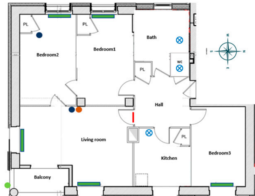
Figure 1. Plan of study apartment: ventilation components and devices locations in each setting and their symbols: ventilation components (■ trickle vent, ⊗ exhaust); symbols of devices: ● NODE, ● NEMO, ● NEMO outdoor, and ■ IAQ sensors.
