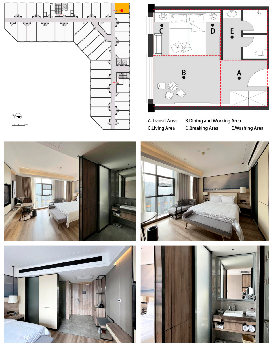
Figure 5. (Top) Typical floor plan of the hotel and spatial layout of the functional zones in the case study hotel room (source: drawings by authors); (Bottom) Photos of the different functional zones in the case study hotel room (source: photographs by research volunteer).
