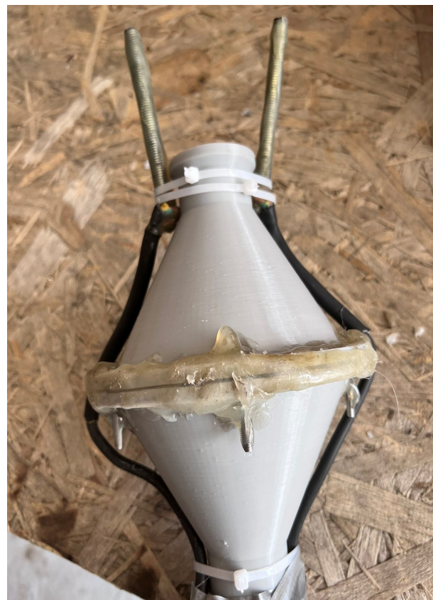
Figure 6. Nozzle with insulated corona electrodes.
