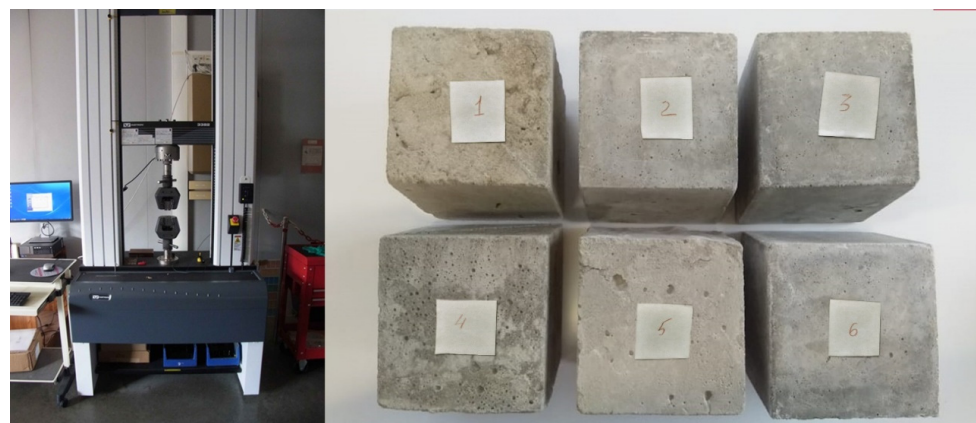
Figure 10. Instron 1100 HDX machine and prototypes.
