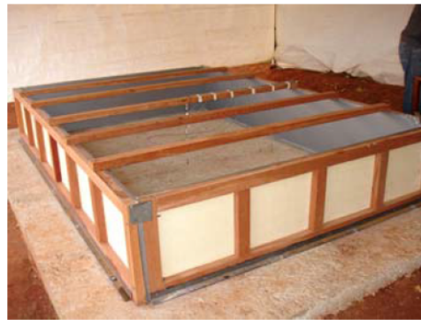
Figure 10. Slab shape tested and monitoring thermometers coupled to the LYNX platform (COPPE/FURNAS).
