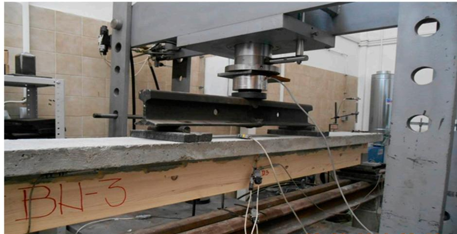
**Figure 9.** Test setup of composite beams BN-series.
