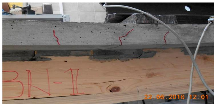
**Figure 21.** Failure of BN-1 beam, crack development in concrete and timber.
