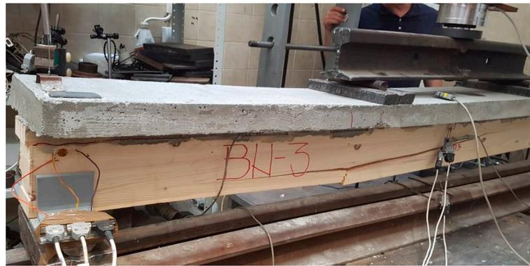
**Figure 22.** Failure of BN-3 beam, crack development in concrete and timber.
