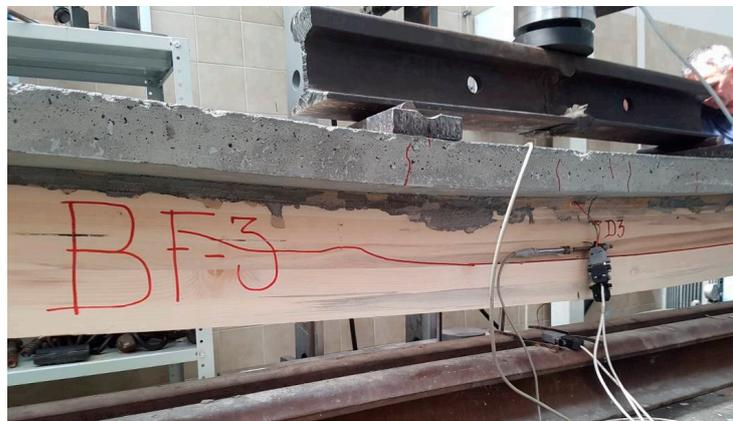
**Figure 20.** Failure of BF-3 beam, crack development in concrete and timber parts.
