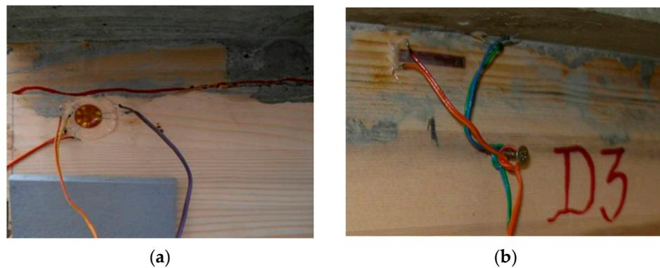
**Figure 10.** (a) Position of rosettes and strain gauges in the zone of support; (b) Position of strain gauges in the middle beam zone in the top side of a timber and bottom side of concrete parts.
