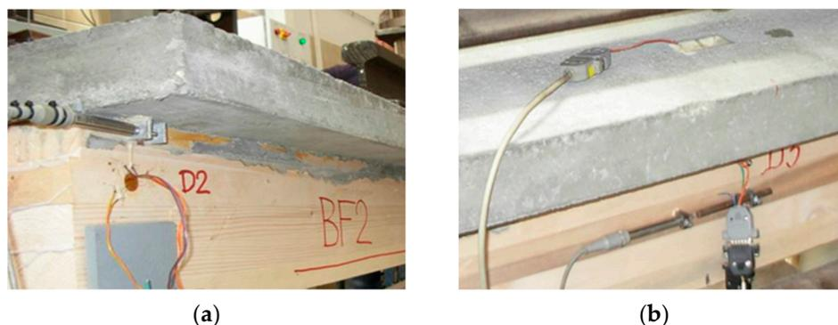
**Figure 11.** (a) Dilatometer in the support zone; (b) Dilatometer in the middle of the beam.
