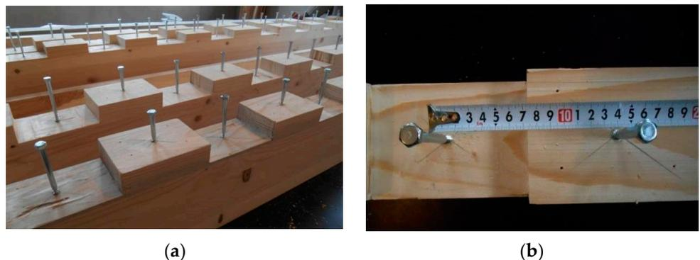
**Figure 3.** (a) System of coupling for BN-beams; (b) Screw + notch reinforced by a screw.
