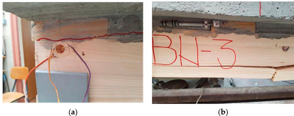
**Figure 23.** (a) Failure of the timber part of the support notch of BN-3 beam; (b) Crack development in concrete and timber in the middle third of the span.
