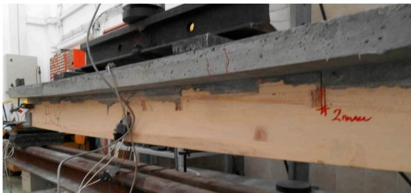
**Figure 24.** Failure of BN-2 beam, crack development in concrete and timber.
