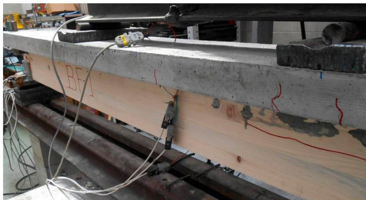
**Figure 18.** Failure of BF-1 beam, cracks development in concrete and timber parts.
