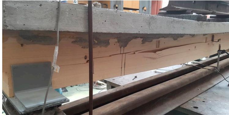
**Figure 19.** Failure of BF-2 beam, crack development in concrete and timber parts.
