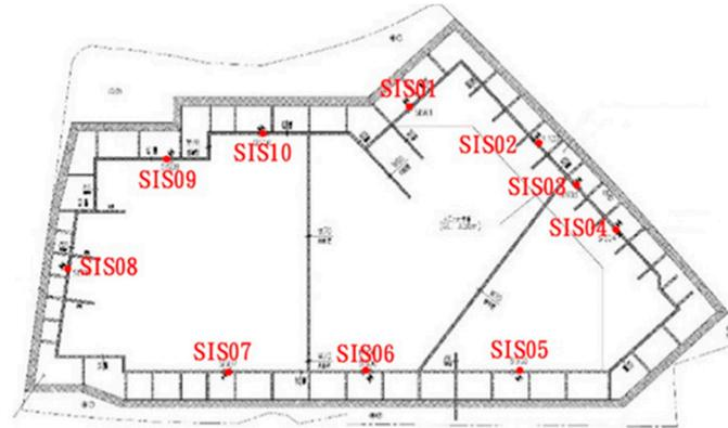
**Figure 13.** Distribution map of inclinometer monitoring locations (where “SISXX” refers to monitoring point number XX).
