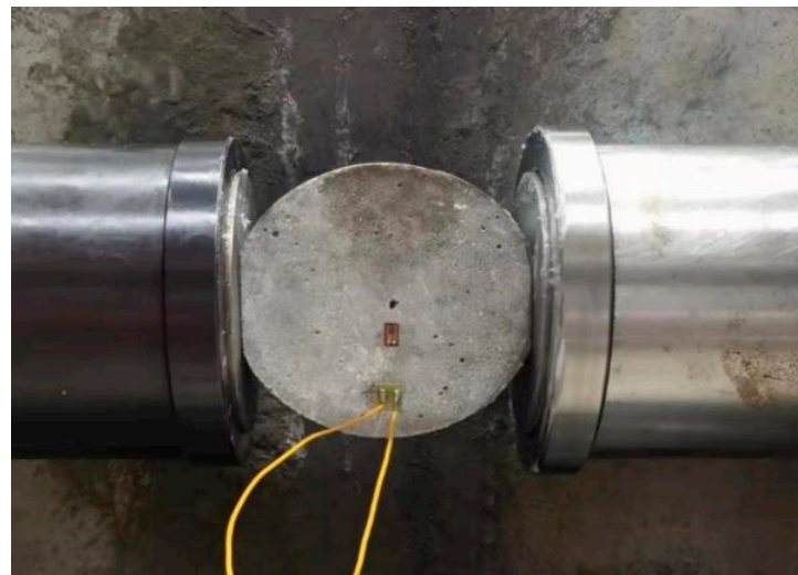
Figure 4. The FBD specimen is placed between two bars.
