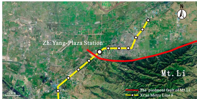
**Figure 3.** Schematic diagram of Metro Line 9 crossing the Piedmont Fault of Li Mountain.
