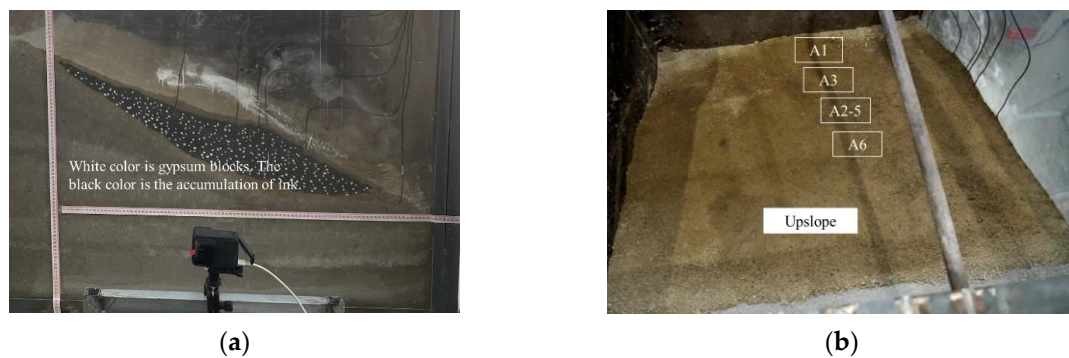
Figure 7. Accumulation slope test model diagram: (a) top view of slope model; (b) front view of slope model.
