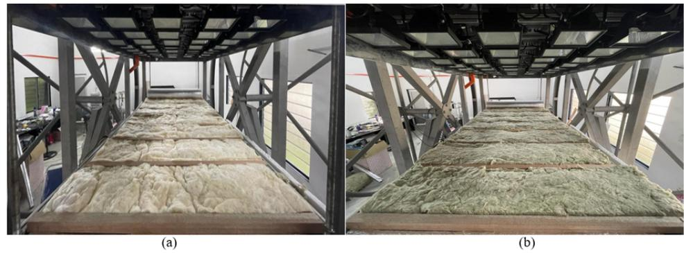
**Figure 8.** (a) Mineral glass wool (50 mm) on top of the reflective foil with battens for roof configurations C1 and C2; (b) stone wool (50 mm) on top of the reflective foil with battens for roof configurations D1 and D2.
