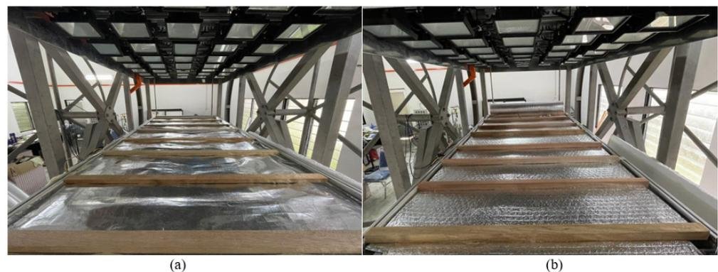
**Figure 7.** (a) Radiant barrier with battens for roof configuration A1 and A2; (b) bubble foil reflective insulation with battens for roof configuration B1 and B2.
