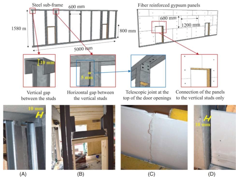
**Figure 5.** (A) Horizontal gap. (B) Door opening. (C) Gypsum panels. (D) Horizontal gap between column and panel. [12].
