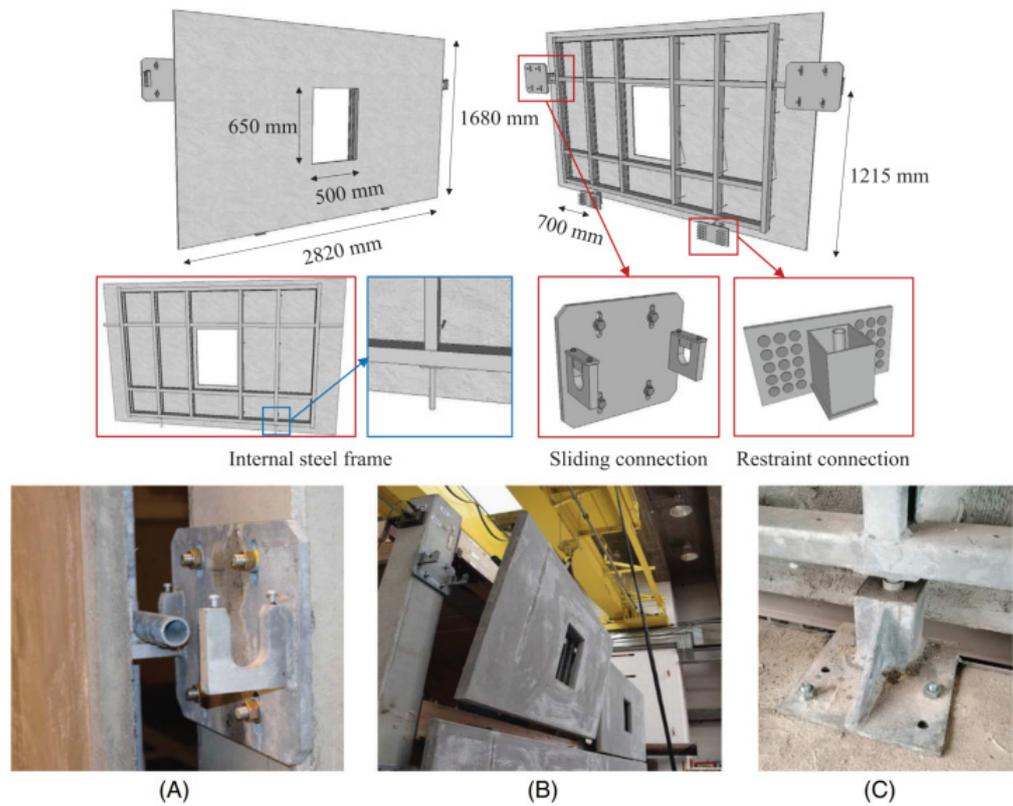
**Figure 7.** (A) Top sliding support. (B) Raising of the GFRC panel. (C) Base support [12].
