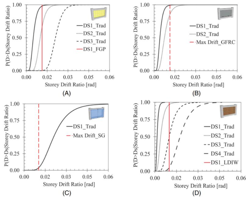
Figure 9. Fragility curves vs. drift ratios. (A) FGP. (B) GFRC. (C) SG. (D) URM [12].
