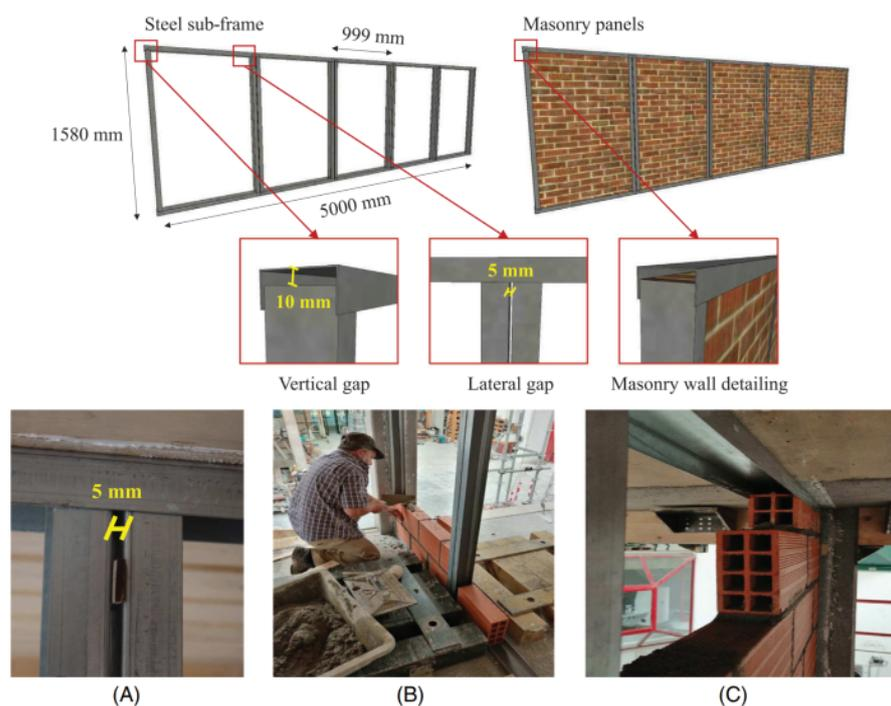
**Figure 6.** Low damage masonry wall. (A) A 5 mm internal gap. (B) Rocking panel. (C) Bricklayers [12].
