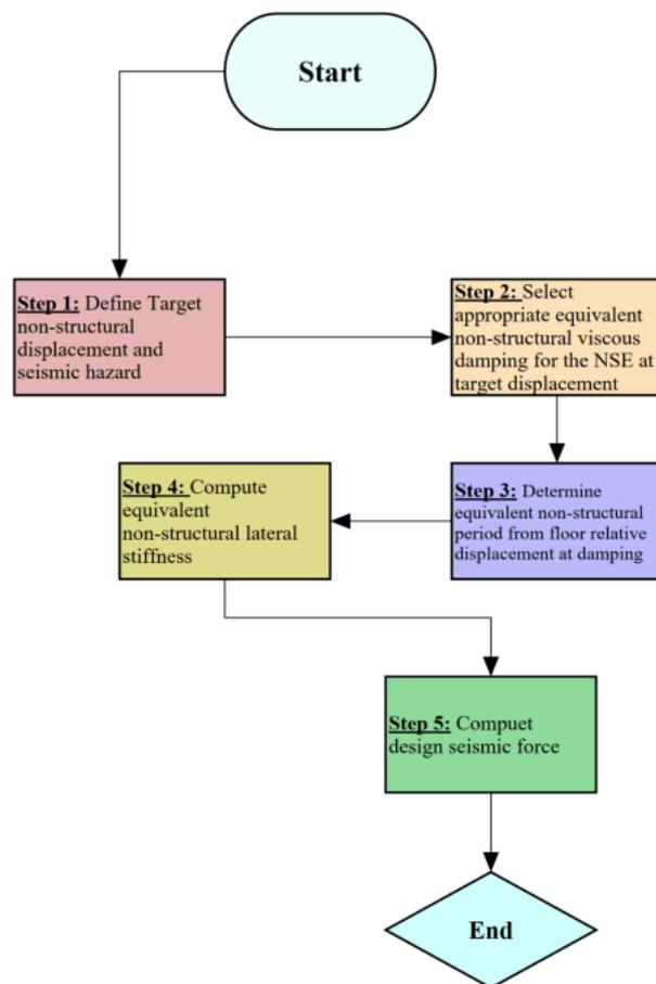
**Figure 11.** Flowchart showing the acceleration-sensitive NSEs direct displacement-based earthquake design.
