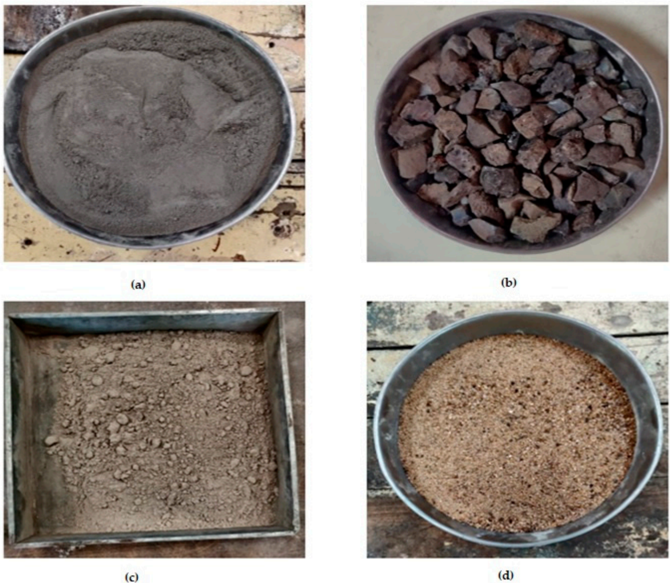
Figure 3. Materials used (a) OPC of grade 53; (b) artificial aggregate; (c) fly ash; (d) fine aggregate.
