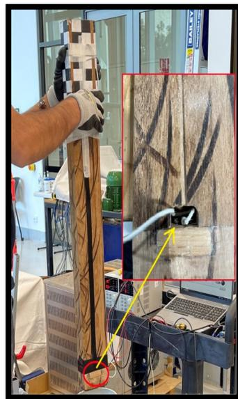
Figure 9. Connection of the accelerometer to the projectile.
