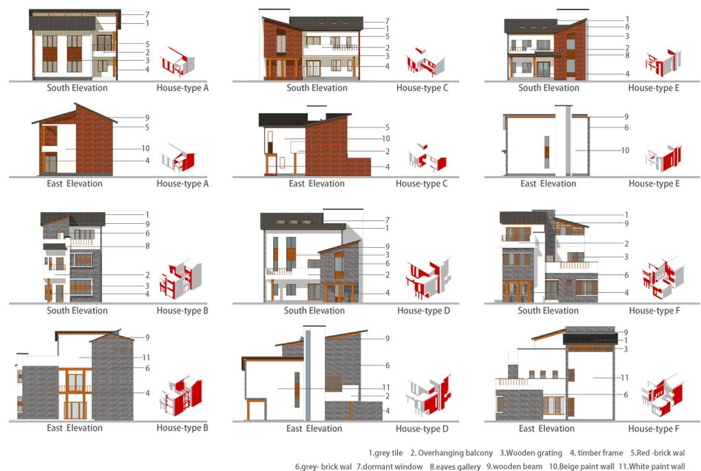
**Figure 8.** The schematic diagram of integrated interfaces for conceptual solutions.
