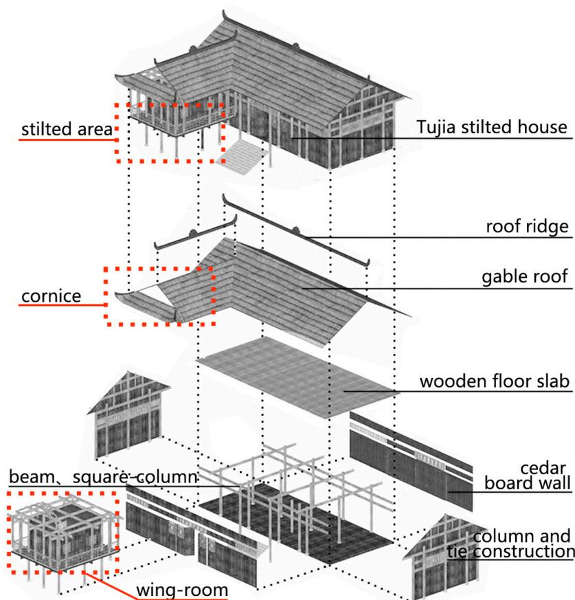
**Figure 4.** Schematic diagram of the structure of a “single-sling” stilted building.
