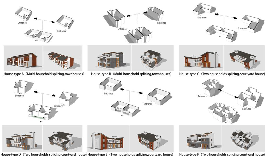
**Figure 11.** Modularization of unit combination.
