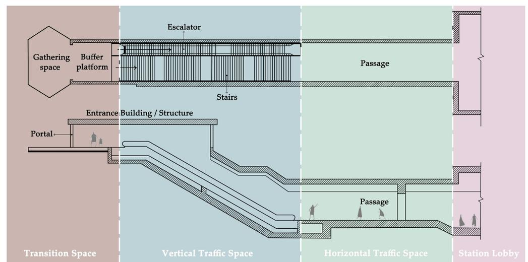
**Figure 1.** Illustration of the typical subway station entrance components.
