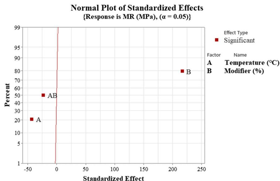
Figure 7. Normal plot for MR of SBS/NS-modified HMA specimens.
