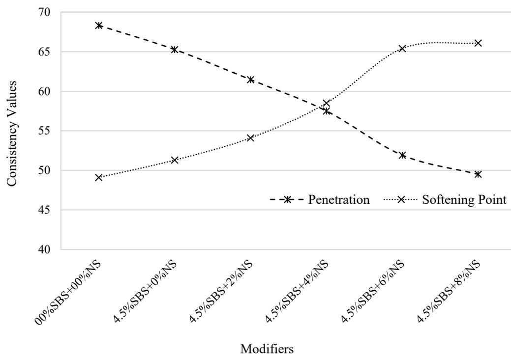
**Figure 3.** Effect of modifiers on consistency of bitumen.
