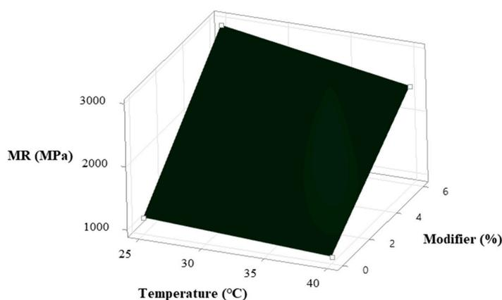
Figure 12. Surface plot for MR of SBS/NS-modified HMA specimens.
