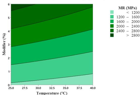
Figure 11. Contour plot for MR of SBS/NS-modified HMA specimens.
