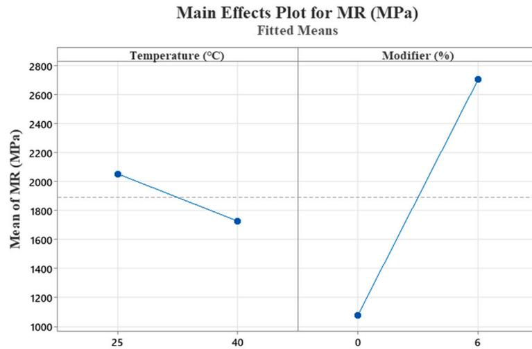
Figure 8. Main effects plot for MR of SBS/NS-modified HMA specimens.
