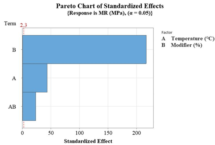
Figure 9. Pareto chart for MR of SBS/NS-modified HMA specimens.
