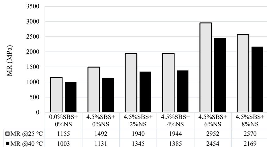
Figure 5. Results of MR test at 25 °C and 40 °C.
