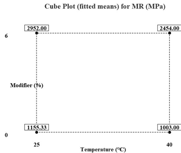
Figure 10. Cube plot for MR of SBS/NS-modified HMA specimens.
