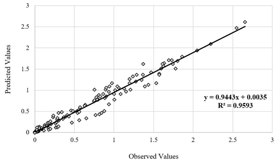
**Figure 13.** Validation data plot of SBS/NS-modified HMA specimens.
