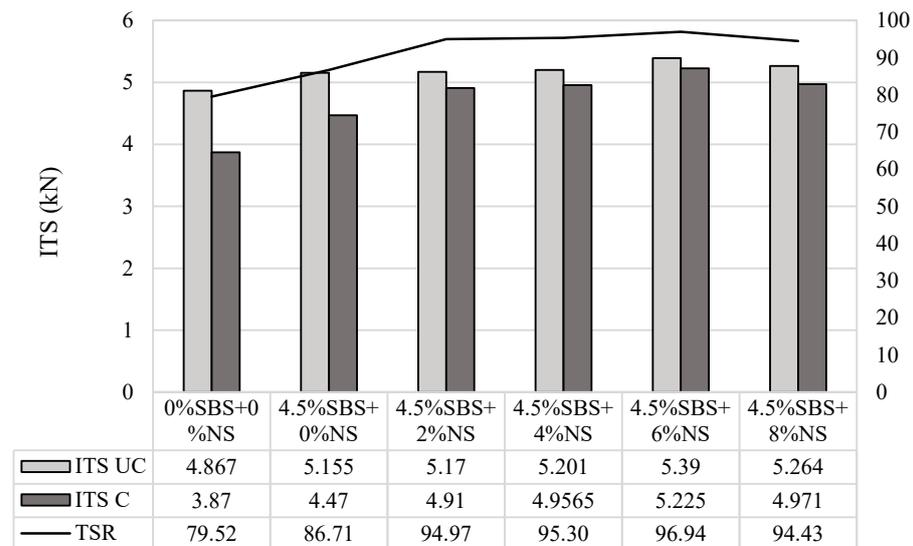
Figure 4. Results of ITS test.
