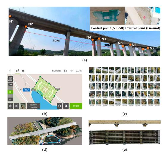
**Figure 13.** Creating scan models using UAVs: (a) control point setup, (b) flight path setup, (c) taking images, (d) creating 3D scan models, (e) dividing into surface scan models.
