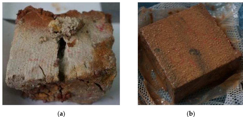
**Figure 10.** Appearances of the two types of rocks after being immersed in water for 24 h: (a) Mudstone interbedded with marl and (b) Sandy mudstone.
