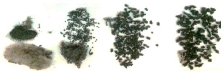
**Figure 15.** Samples of crumb rubber used in manufacturing of tire-aggregate-concrete BRBs [123].
