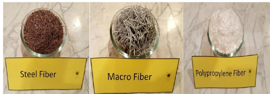
**Figure 13.** Samples of fibers used in Fiber-reinforced-concrete BRBs. (Reprinted with permission from Ref. [121]. Copyright 2018 Elsevier.)
