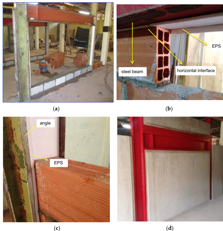
Figure 10. Constructing the experimental model: (a) steel frame overview; (b) masonry placement in relation to the horizontal joint; (c) masonry placement in relation to the vertical joint; (d) appearance of the model before treating the joints between the masonry and the steel beam.
