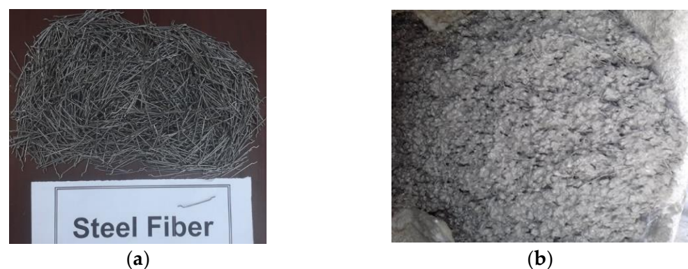
Figure 1. (a) steel fibers (b) high-strength concrete with fibers during mixing.
