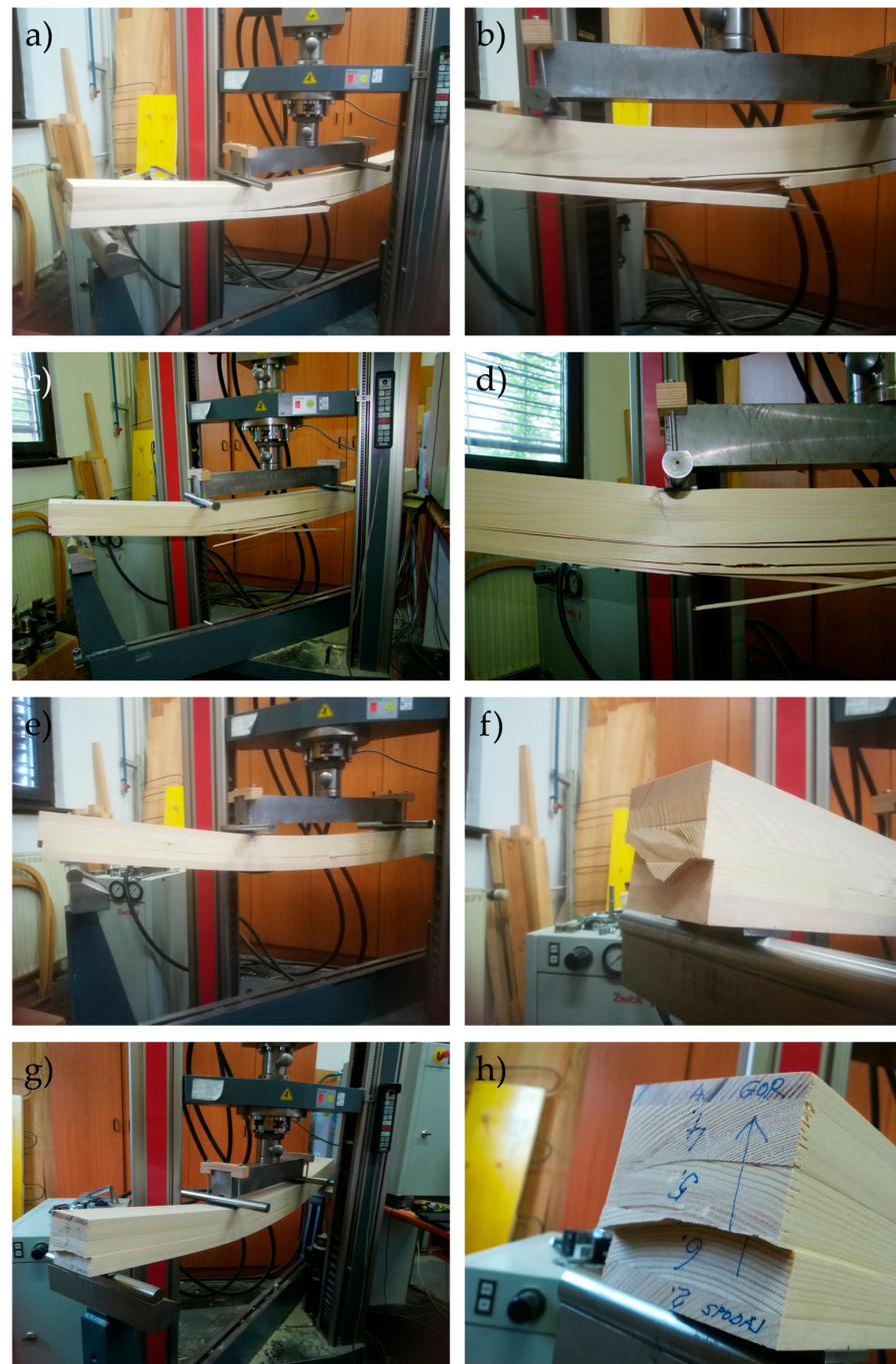
Figure 6. Beams after four-point bending tests. (a) Beam beech 2; (b) bending failure of beam beech 2; (c) beam spruce 2; (d) bending failure of beam spruce 2; (e) beam Hybrid 20-20 1; (f) shear failure of beam Hybrid 20-20 1; (g) beam Hybrid 11-11 2; (h) shear failure of beam Hybrid 11-11 2.
