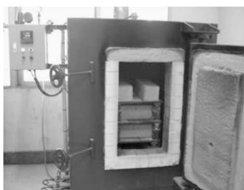
Figure 1. Specimens in oven chamber according to ASTM E119-98.
