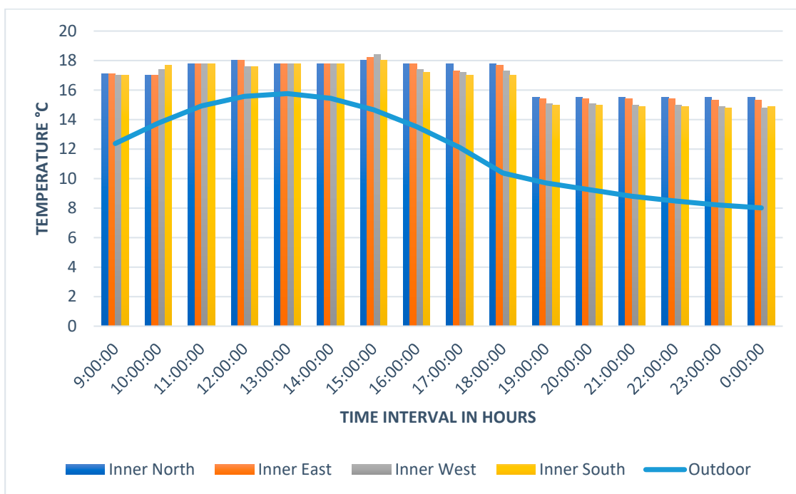
Figure 16. Variation in surface temperature of envelopes in bedroom 7.
