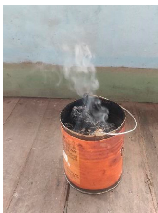
Figure 13. Smoke tracer for determination of wind direction in the main hall.
