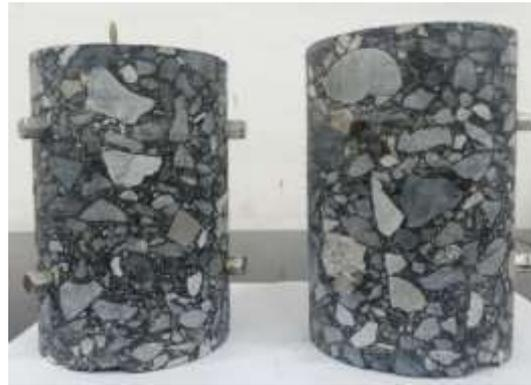
Figure 6. Standard specimen after core cutting.
