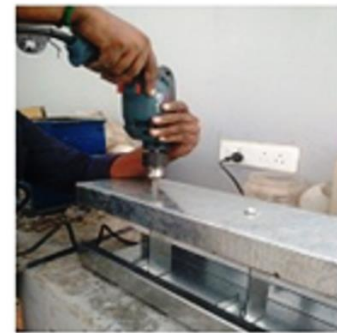
(b) SCS beam mould (using CFS with STS) making process
