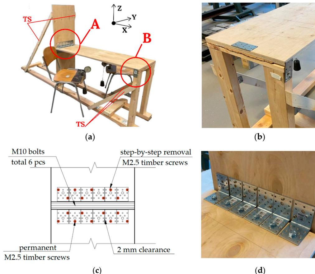
**Figure 2.** Investigated object: (a) stend for modelling semirigid panel-to-panel structural joints of multi-storey buildings, where A is the investigated moment joint of plywood panels, B is a free-end connection of a horizontal plywood panel, and TS are additional timber supports used to ensure stability and reduce unwanted movements of the stend; (b) free-end connection of horizontal plywood panel; (c,d) investigated moment joint of plywood panels.
