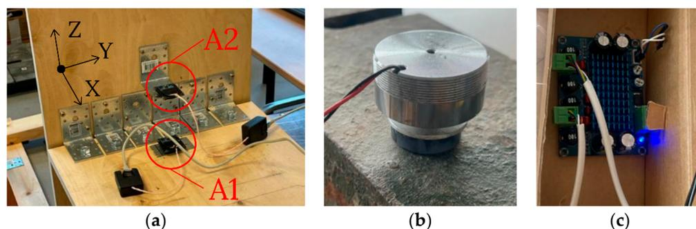
**Figure 4.** (a) The coaxial placement of the accelerometers A1 and A2 on either side of the investigated timber joint; (b) the electrodynamic actuator for generating sweep signals; and (c) the custom-built board.
