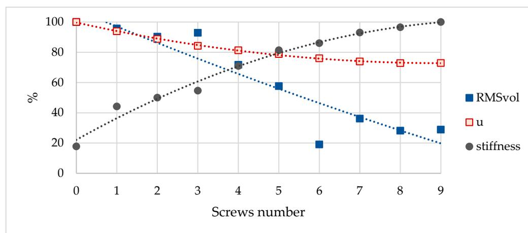
**Figure 7.** Calculated volume root mean square (RMS<sub>vol</sub>) and experimental displacements (u) and rotational stiffness of the investigated joint values for various grades of joint degradation as a percentage from the RMS<sub>vol</sub>, u, and stiffness maximal values.
