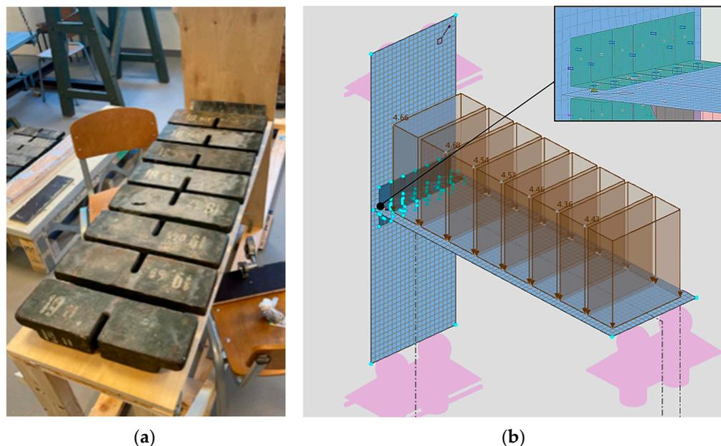
**Figure 3.** (a) The placement of the steel pieces during the loading of the stand; (b) the numerical model of the panel-to-panel structure with modelled screws.
