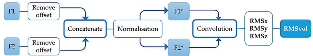
**Figure 5.** Post-processing scheme of the collected specimen raw response data F1 and F2 from the A1 and A2 accelerometers to the processed specimen response signals F1\* and F2\* for further similarity comparison using convolution and root mean square (RMS).
