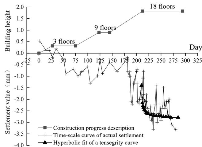
**Figure 16.** Track settlement-versus-time curve.
