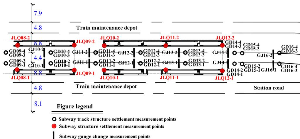
Figure 13. Measurement point layout plan (I).
