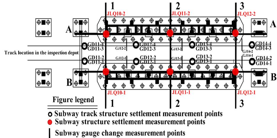
Figure 17. Contrast measurement line positions.
