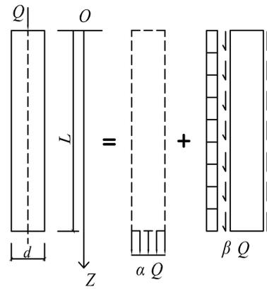
Figure 4. Schematic diagram of single pile load in Mindlin’s solution.
