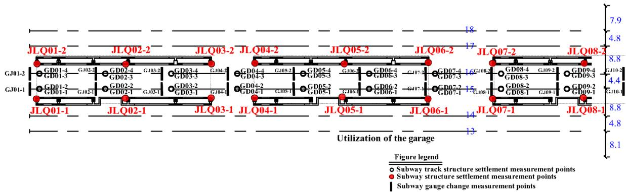
Figure 14. Measurement point layout plan (II).
