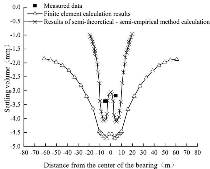
Figure 18. Measured line 2–2 settlement trend and observed values.
