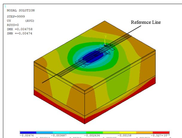
Figure 9. Calculation results of the additional settlement of upper load (m).
