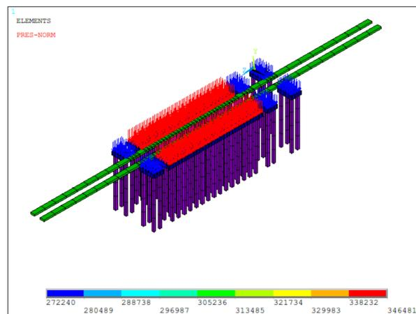
Figure 8. Foundation and load application (m).
