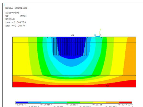
**Figure 10.** Settlement contour of the maximum settlement section along the line road direction (m).
