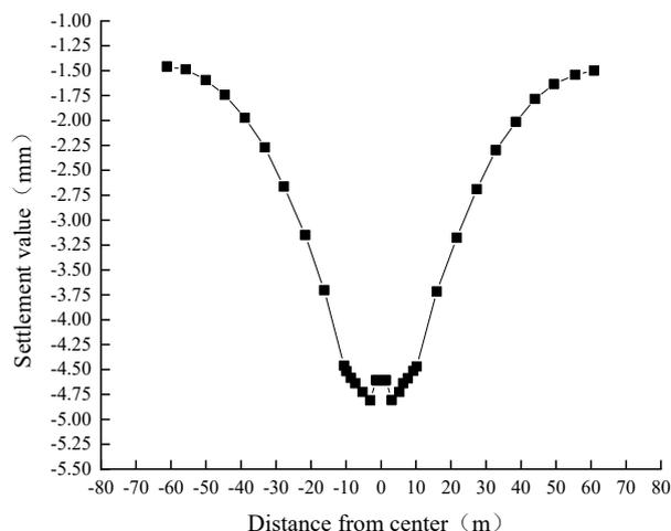
**Figure 11.** Settlement curve of the reference line position.
