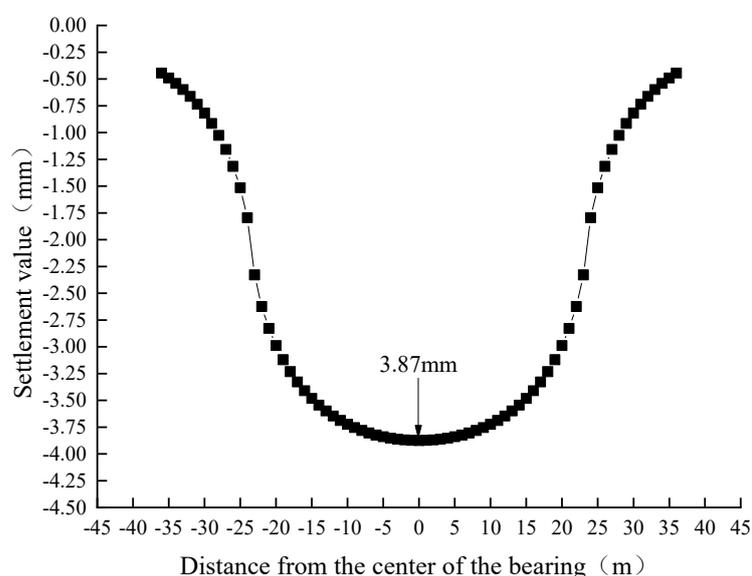
**Figure 6.** Settlement curve of the rail track.
