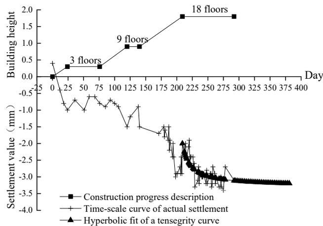
**Figure 15.** Foundation settlement versus time curve.
