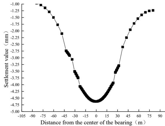
Figure 12. Track position settlement curve.
